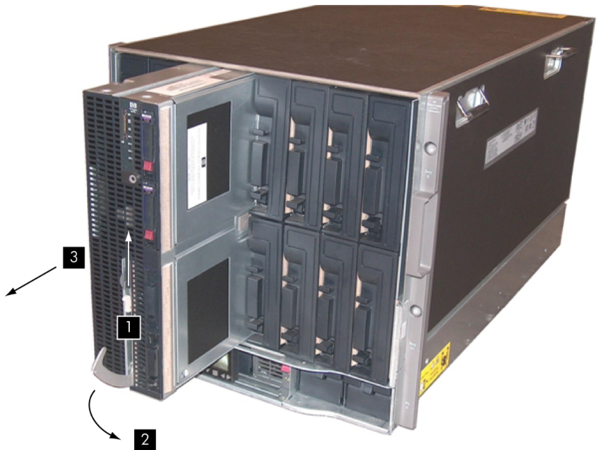
Figure 41 Removing the Server Blade from the Enclosure
