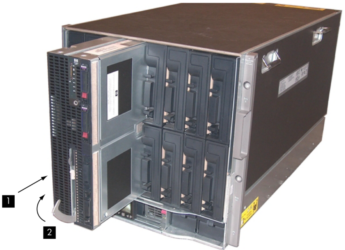
Figure 42 Installing the Server Blade into the Enclosure
