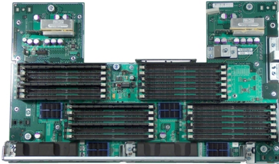
Figure 49 Memory Mezzanine Board
