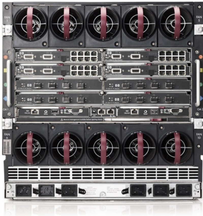
Figure 32 Interconnect Modules on the Rear of the Server Blade Enclosure
