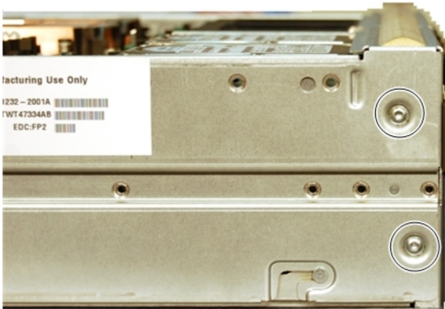
Figure 58 Removing the Front Panel Housing Screws
