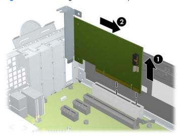
**c.** If you are removing a PCI Express x16 card, pull the retention arm on the back of the expansion socket away from the card and carefully rock the card back and forth until the connectors pull free from the socket. Pull the expansion card straight up from the socket then away from the inside of the chassis to release it from the chassis frame. Be sure not to scrape the card against the other components.
