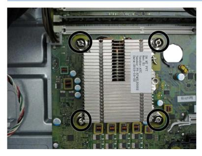
5. Lift the heat sink from atop the processor.
