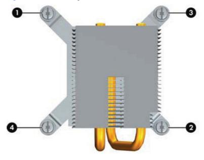
**6.** After loosening the Torx T15 screws **(1)**, lift the heat sink from atop the processor **(2)** and set it on its side to keep from contaminating the work area with thermal grease.
