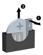
NOTE: After the battery has been replaced, use the following steps to complete this procedure.
