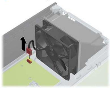
6. Press the tabs that secure the fan assembly to the front of the chassis (1).
