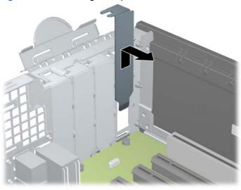
**b.** If you are removing a standard PCI card or PCI Express x1 card, hold the card at each end, and carefully rock it back and forth until the connectors pull free from the socket. Pull the expansion card straight up from the socket (1) then away from the inside of the chassis to release it from the chassis frame (2). Be sure not to scrape the card against the other components.
