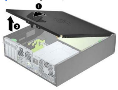
To install the access panel, reverse the removal procedure.
