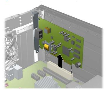
**c.** If you are removing a PCI Express x16 card, pull the retention arm on the back of the expansion socket away from the card and carefully rock the card back and forth until the connectors pull free from the socket. Pull the expansion card straight up from the socket then away from the inside of the chassis to release it from the chassis frame. Be sure not to scrape the card against the other components.
