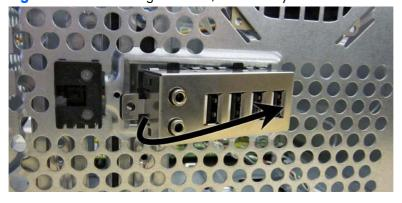
8. Pull the assembly away from the computer while threading the wires through the hole in the front of the chassis.
