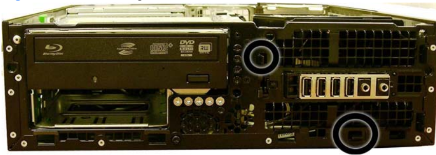
Figure 7-54 Removing the front fan
