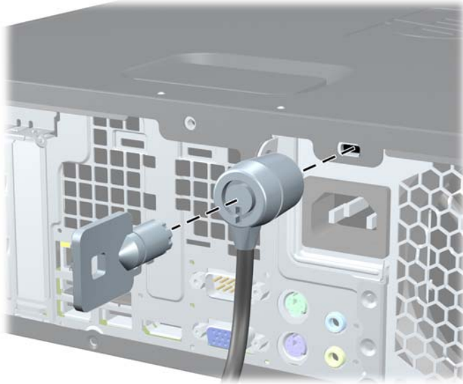
Figure 7-3 Installing a Cable Lock
