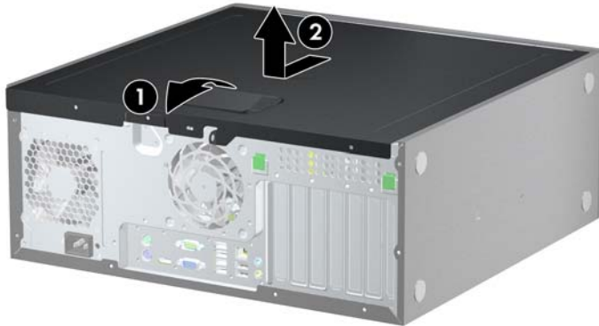
Figure 6-11 Removing the Computer Access Panel
