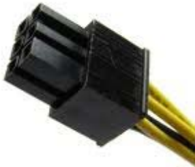
Figure 6-14 6-pin power connector
