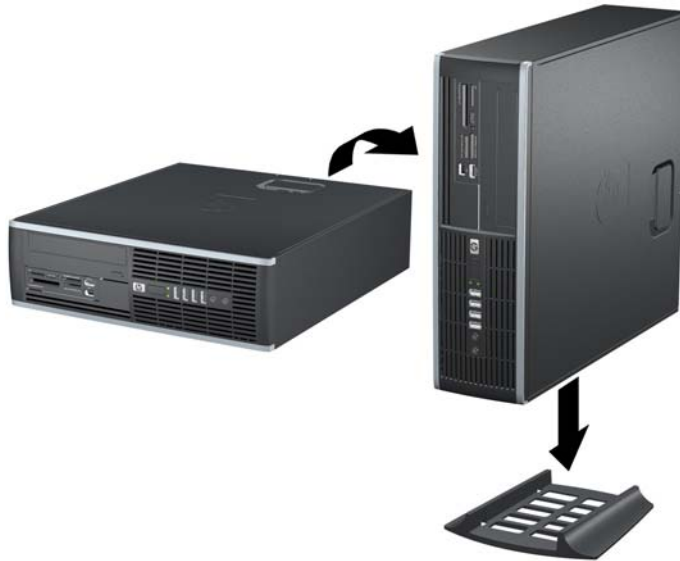
Figure 7-65 Changing from Desktop to Tower Orientation
