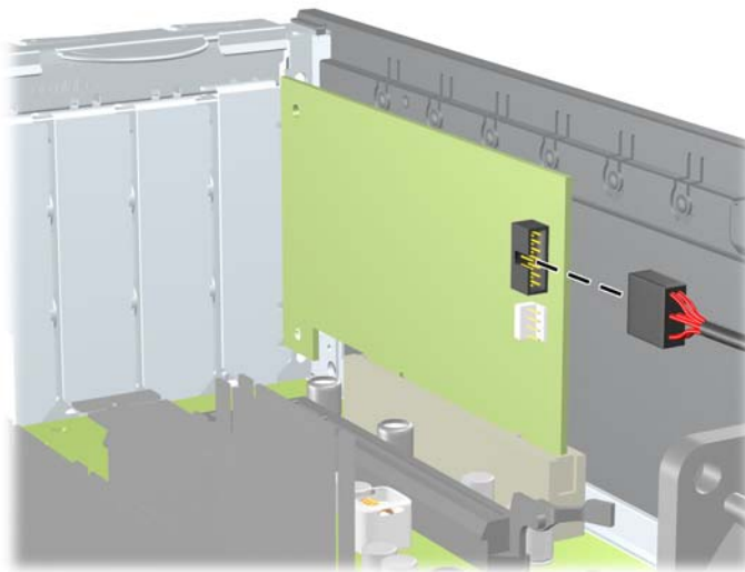
Figure 7-36 Disconnecting the Media Card Reader 1394 Cable
