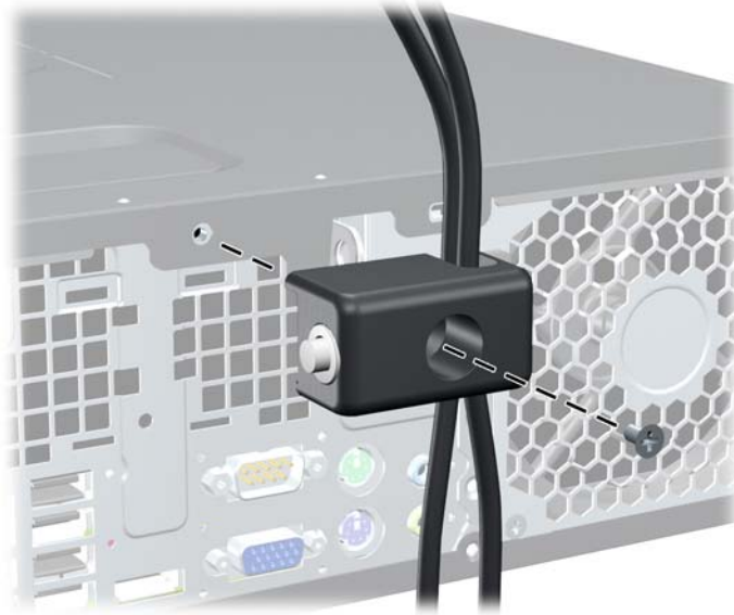
Figure 7-7 Attaching the Lock to the Chassis
