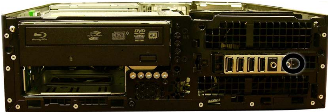
Figure 7-56 Removing the front I/O, power switch/LED assembly screw
