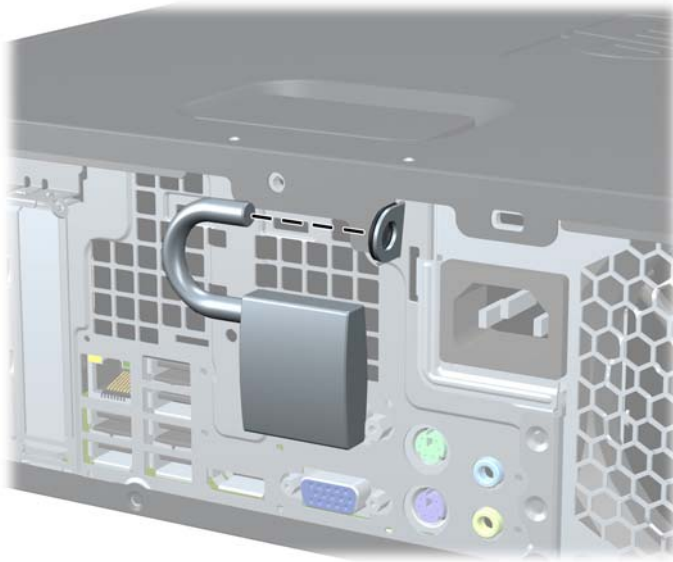
Figure 7-4 Installing a Padlock
