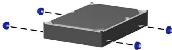
Figure 7-43 Installing Hard Drive Guide Screws
