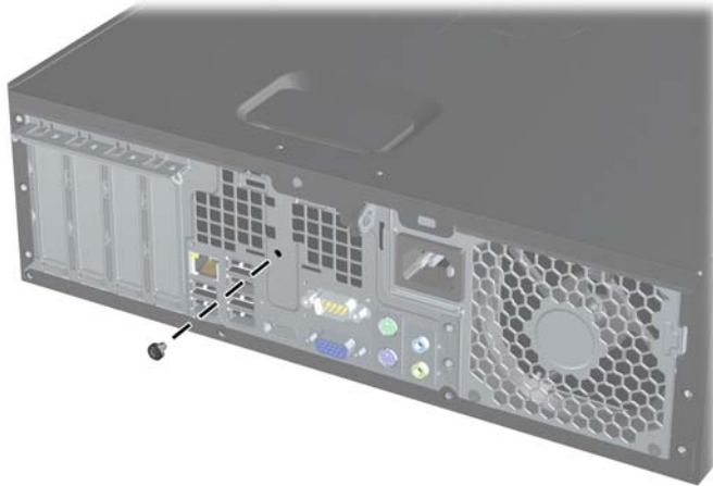
Figure 7-2 Removing the Smart Cover Lock Screw
