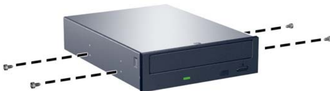
Figure 7-31 Installing Guide Screws in the Optical Drive
