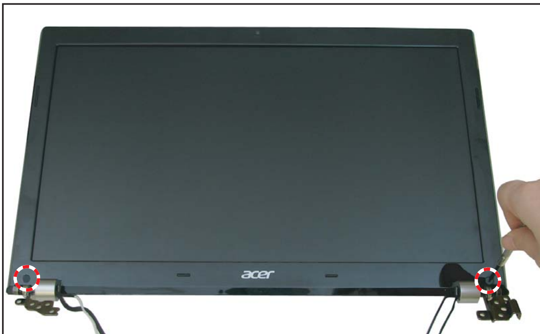
Figure 3:132. Removing the LCD Bezel (1 of 3)
