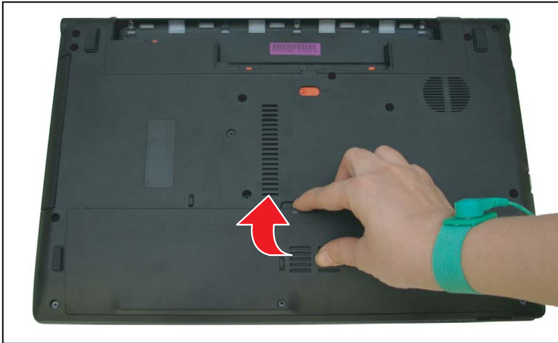
Figure 3:11. Installing the Base Door
