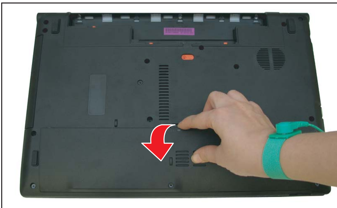
Figure 3:9. Removing the Base Door
