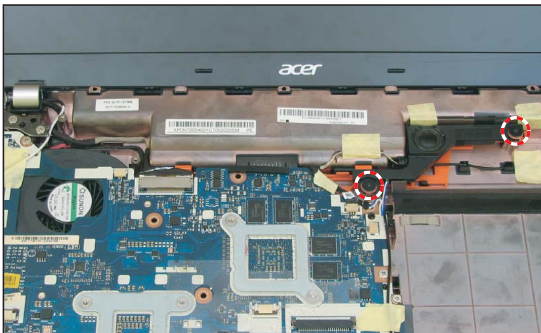
Figure 3:94. Securing the Right Speaker Screws
