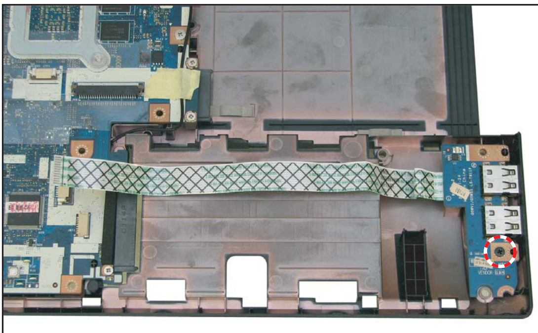
Figure 3:100. Removing the USB Module Screw
