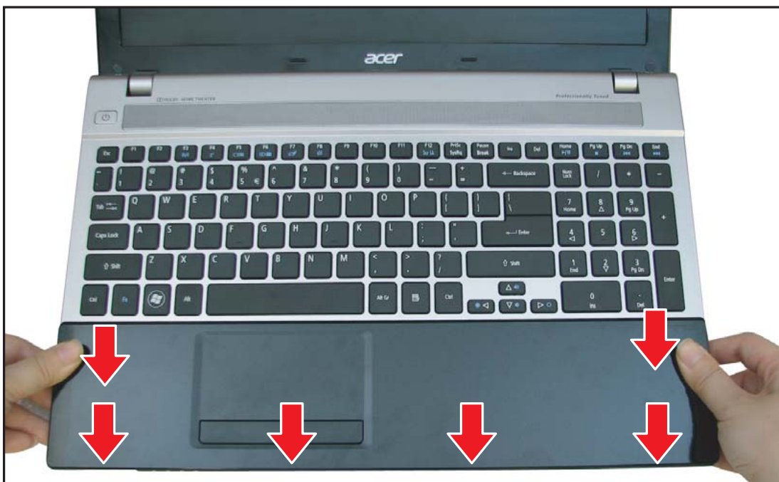
Figure 3:46. Installing the Palm Rest (2 of 2)
