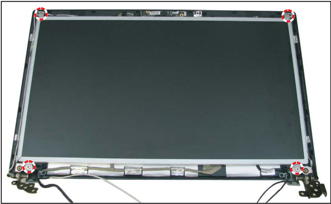
Figure 3:156. Securing the LCD Panel Screws
