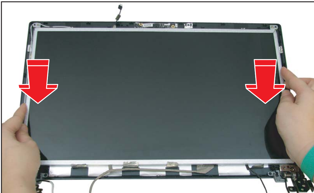
Figure 3:153. Installing the LCD Panel
