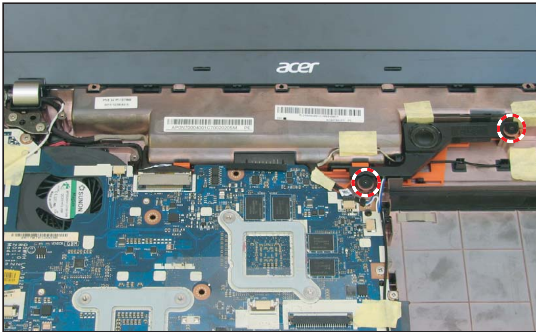
Figure 3:91. Removing the Right Speaker Screws
