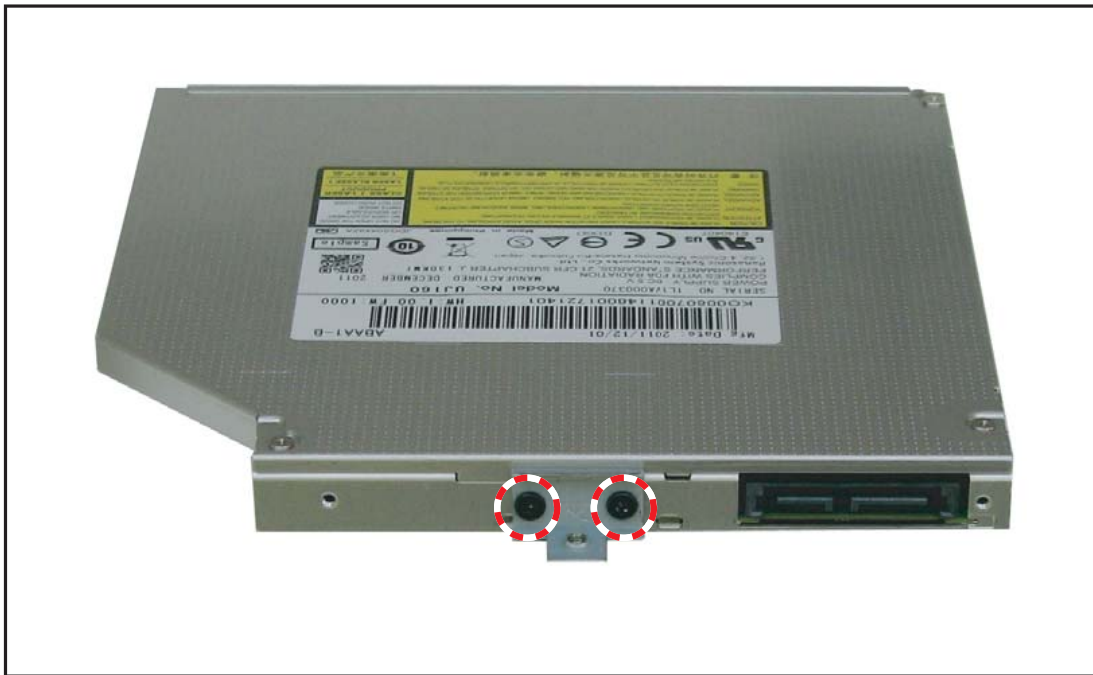
Figure 3:19. Attaching the ODD Bracket
