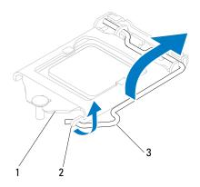
processor cover 2 tab 3 release lever
