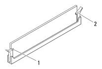
1 cutouts (2) 2 securing clips (2) (snapped in position)
