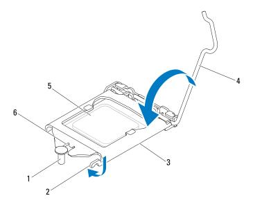
1 alignment post 2 tab 3 processor cover 4 release lever 5 processor 6 processor cover notch
