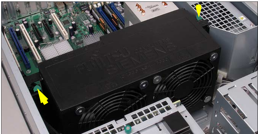
Figure 55: Removing the standard fans
