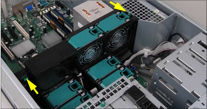
Figure 20: Removing the processor fan holder
