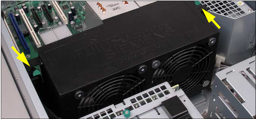
Figure 25: Installing the standard fans
