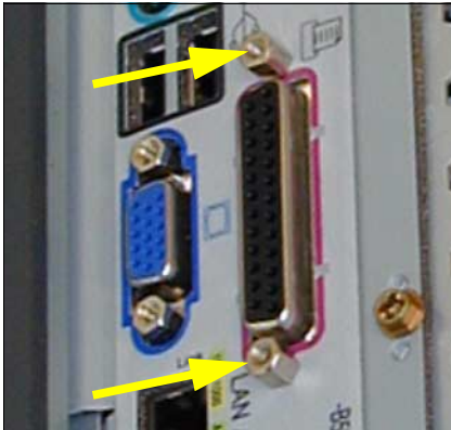
Figure 53: Fastening the plug connector at the rear of the housing
