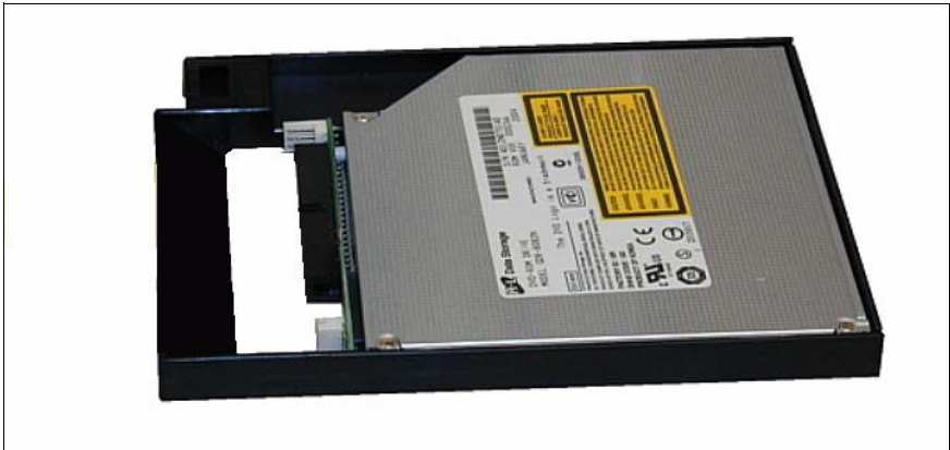
Figure 33: Installing the CD-DVD-ROM drive in the mounting frame
