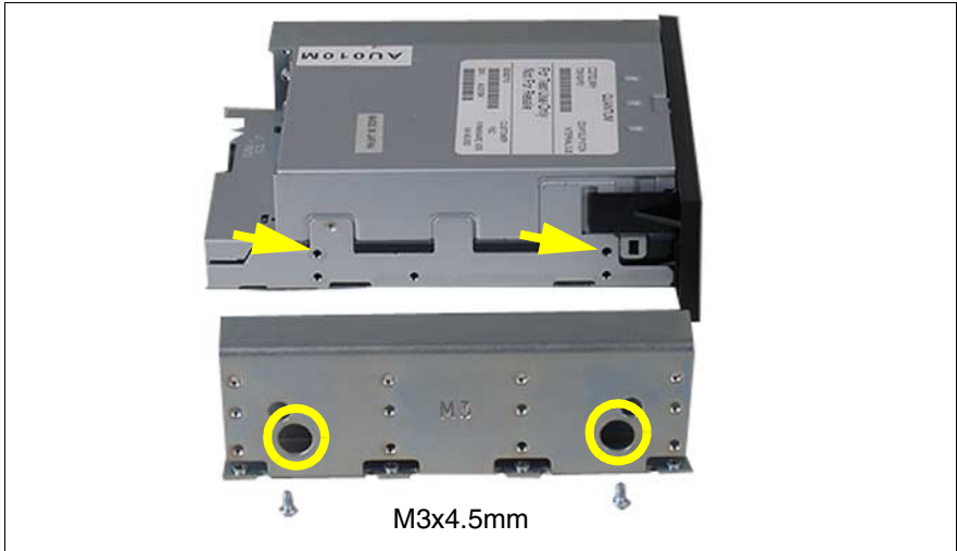
Figure 41: Attaching the frame - magnetic tape drive DAT72
