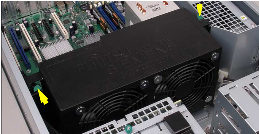
Figure 16: Removing the standard fans
