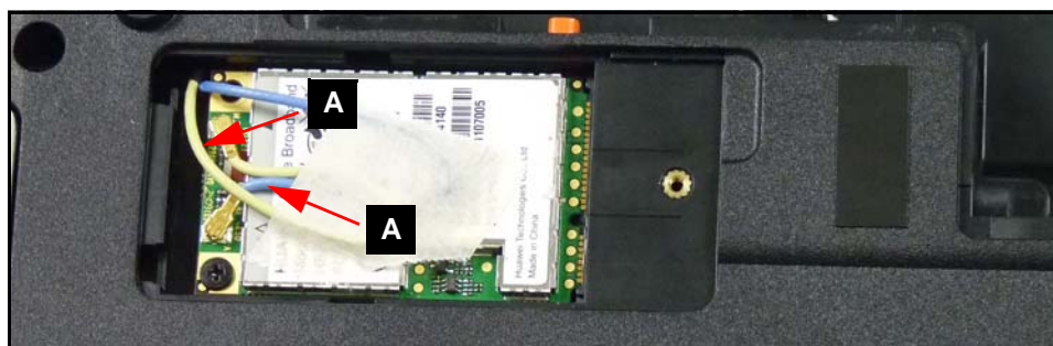
Figure 3-54. 3G Module Cables
