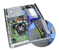
7. Pry the thermal sensor away from the chassis front and remove.
