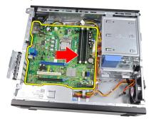
11. Remove the system board from the chassis.
