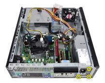
**9.** Push in on the blue release tab beside the power supply, and slide the power towards the front of the computer.
