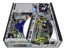
6. Disconnect the 24-pin power cable from the system board.
