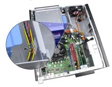
5. Press down the speaker-securing tab and slide the speaker upwards to remove it.
