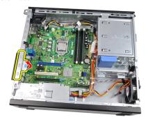
9. Remove the screws that secure the system board to the chassis.
