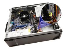
5. Unthread the thermal-sensor cable from the chassis clips.
