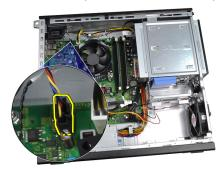
5. Unthread the system-fan cable from the chassis clips.
