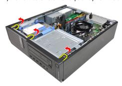
**4.** Rotate the bezel away from the computer to release the hooks on the opposite edge of the bezel from the chassis.
