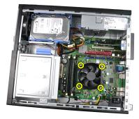
Lift the heat sink assembly upwards, and remove it from the computer. Lay the assembly with the fan facing downwards, and with the thermal grease facing upwards.
