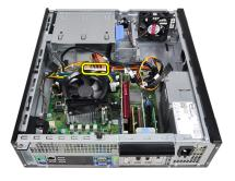
7. Unthread the 24-pin power cable from the chassis clip.
