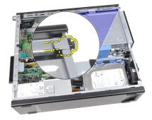
6. Slide the power-switch cable out through the front of the computer.
