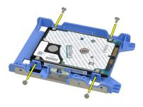
8. Release the screws that secure the 2.5 inch hard drive to the top of the hard-drive bracket.
