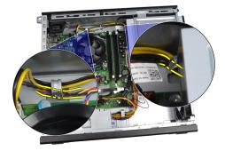
**6.** Slide the four grommets inward and through the slots in the front of the computer.
