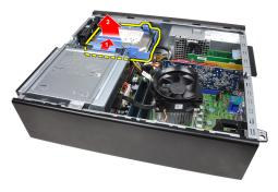
Flex the hard-drive bracket and then remove the single 3.5 inch hard drive or two 2.5 inch hard drives from the bracket.
