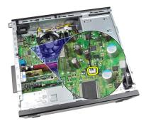
4. Unthread the thermal-sensor cable from the chassis clip.
