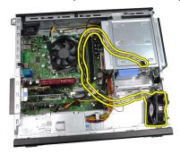
8. Pry up and remove the four grommets from the system fan.
