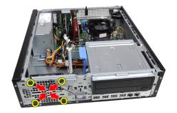
7. Lift and remove the system fan out of the computer.
