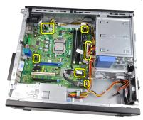
Lift and release the expansion-card latch to gain access to the screws securing the system board.
