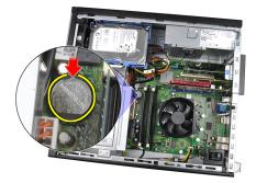
4. Lift the coin-cell battery out of the computer.
