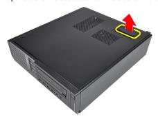
3. Lift the cover upward to a 45-degree angle and remove it from the computer.
