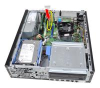
**6.** Lift the PCI expansion card (if any) up and out of its connector and remove it from the computer.
