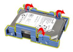
Turn over the hard-drive bracket and release the screws that secure the 2.5 inch hard drive to the underside of the bracket.
