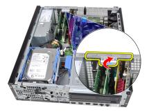
4. Pull the release lever away from the PCIe x16 card to release the securing tab from the dent in the card. Then, ease the card up and out of its connector and remove it from the computer.
