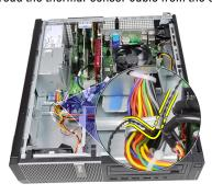
5. Pry the thermal sensor away from the power supply and remove from the chassis.
