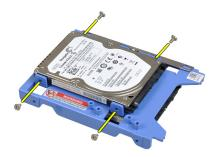
Flex the hard-drive bracket and then remove the two 2.5 inch hard drives from the bracket.
