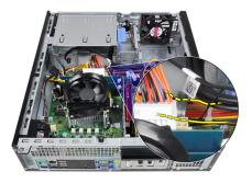
8. Remove the screws that secure the power supply to the back of the computer.
