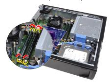
4. Lift the memory modules out of the connectors on the system board.
