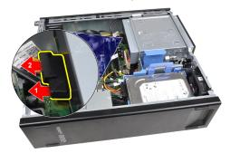
5. Slide up the optical-drive latch and then push the optical drive from the back towards the front of the computer.
