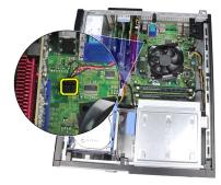
Slide the intrusion switch toward the chassis bottom and remove it from the system board.
