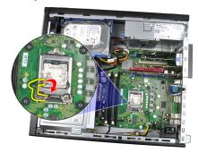
8. Lift the processor to remove it from the socket and place it in an antistatic package.
