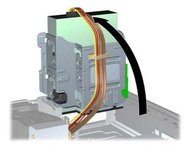
Rotate the power supply to its upright position. The hard drive is located beneath the power supply.
