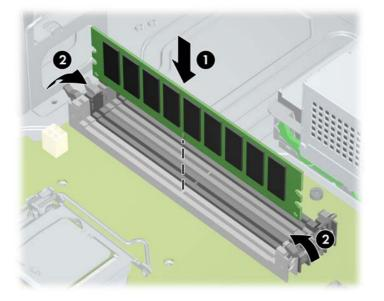
Figure 5-48 Opening DIMM socket levers
