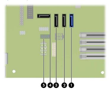
Figure 5-9 System board drive connections
