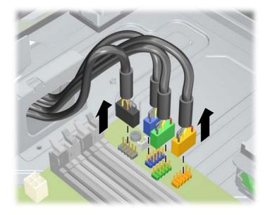
Carefully guide the cables through the chassis openings (1), as shown in the following figure.
