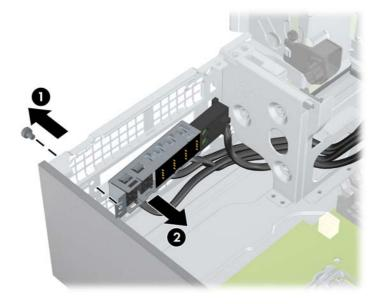
Disconnect the front panel I/O device assembly cables from the system board as shown below.
