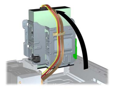
Disconnect the power cable (1) and data cable (2) from the rear of the optical drive.
