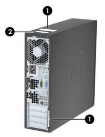
In general, the serial number labels can be found on the top panel or on the side of the computer and at the rear of the computer (your computer may look different). Keep this number available when contacting customer service for assistance.
