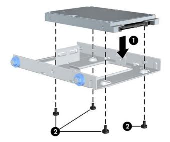
9. Align the guide screws with the slots on the chassis drive cage, press the hard drive down into the bay, then slide it back until it stops and locks in place.
