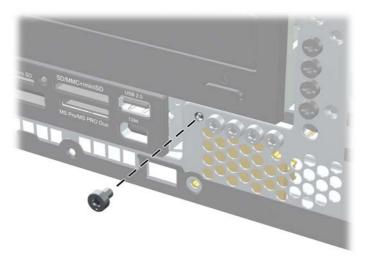
Figure 5-5 Retrieving the Front Bezel Security Screw
