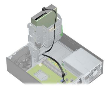
9. If necessary, route the data cable through the cable guides. There are two cable guides that keep the data cable from being pinched by the drive cage when raising or lowering it. One is located on the bottom side of the drive cage. The other is located on the chassis frame under the drive cage. Ensure that the data cable is routed through these guides before connecting it to the optical drive.
