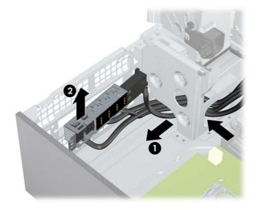
8. Carefully lift the front panel I/O device assembly and cables from the chassis (2).
