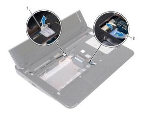
1 power button board cable connector 2 touch pad cable
