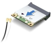
$\Delta$  CAUTION: When the Mini-Card is not in the computer, store it in protective antistatic packaging. For more information, see "Protecting Against Electrostatic Discharge" in the safety information that shipped with your computer.
