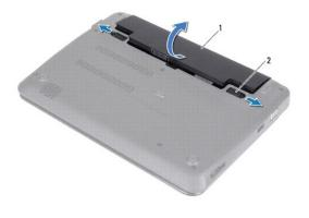
1 battery 2 battery release latches (2)
