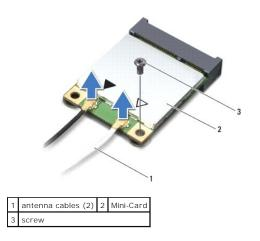
7. Remove the screw that secures the Mini-Card to the system board.
