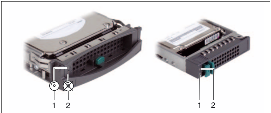
Figure 25: Indicators on the 3.5 inch and 2.5 inch HDD modules
