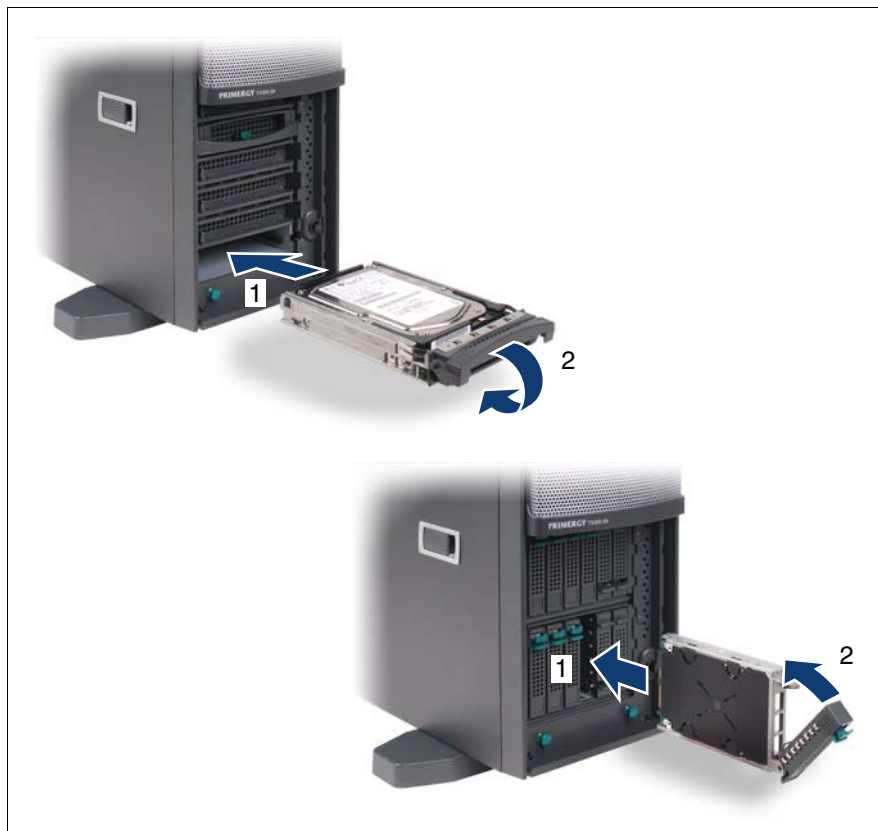
Figure 35: Installing the 3.5-inch and 2.5-inch HDD modules
