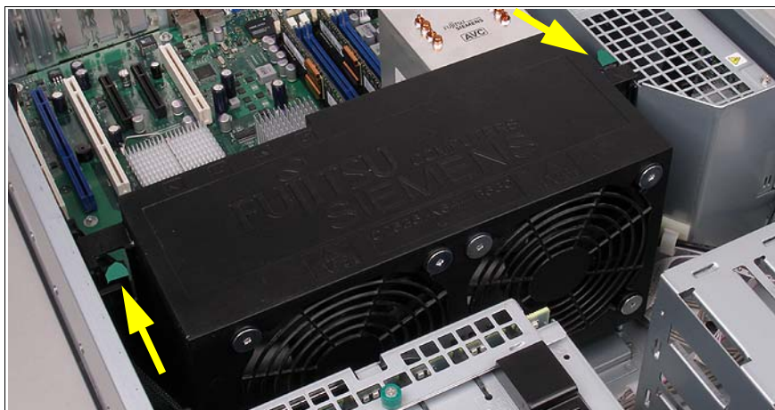
Figure 45: Installing the standard fan module
