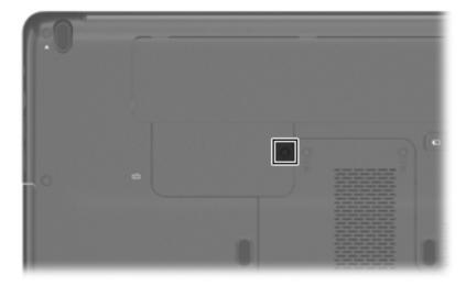
Where used: 1 screw that secures the WLAN cover to the base enclosure
