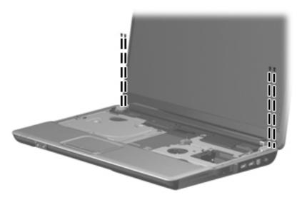
Where used: 4 screws that secure the display hinges to the computer
