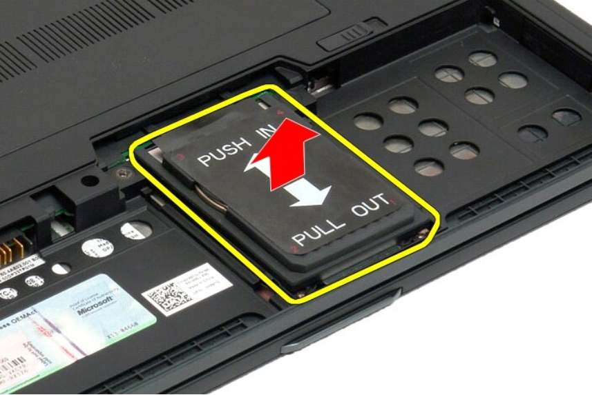
6. Remove the hard drive from the Tablet-PC.
