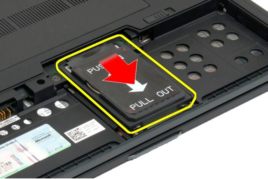
6. Remove the hard drive from the Tablet-PC.
