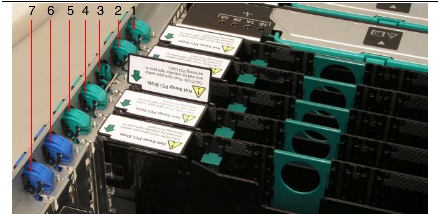
Figure 31: PCI slots with and without hot-plug functions
