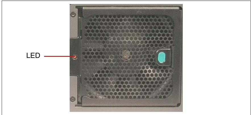
Figure 17: Fan status indicator (right fan unit)
