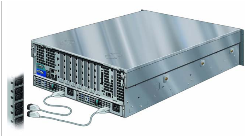
Figure 13: Connecting the server to the mains voltage
