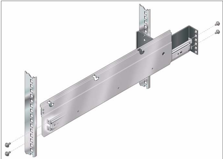
Figure 6: Mounting the telescopic rails into the PRIMECENTER Rack
