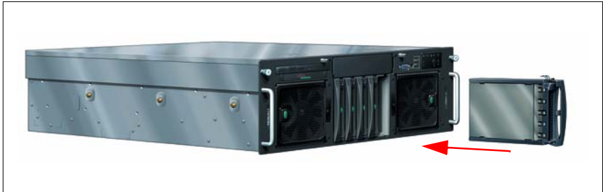
Figure 26: Installing the HDD module
