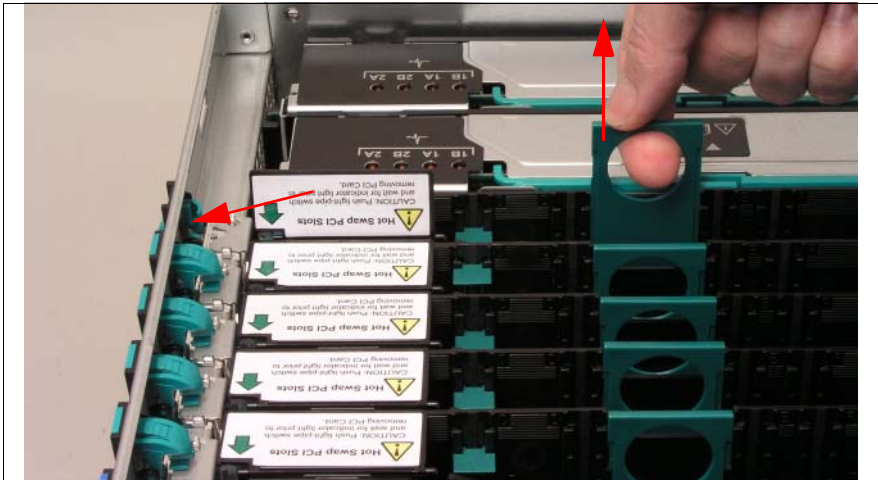
Figure 33: Unlocking a PCI board and removing it by its pull-out aid
