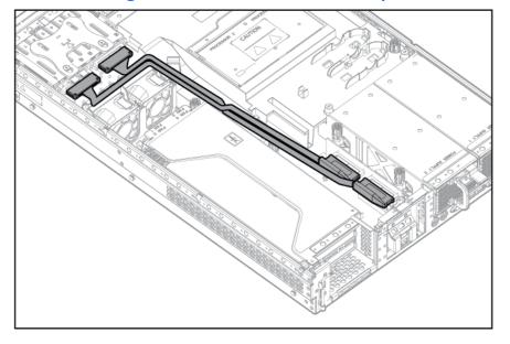
PCI SAS cabling to an optional expansion board controller
