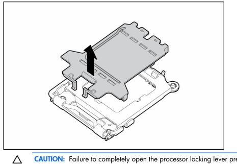
**CAUTION:** Failure to completely open the processor locking lever prevents the processor from seating during installation, leading to hardware damage.
