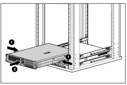
**b.** Slide the server fully into the rack.
