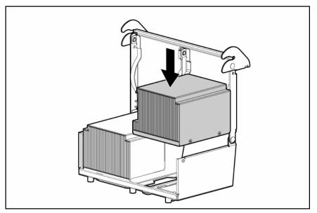
14. Close the heatsink retaining bracket.
