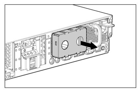
3. Slide the power supply into the power supply bay.
