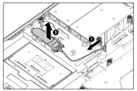
5. Remove the air baffle.
