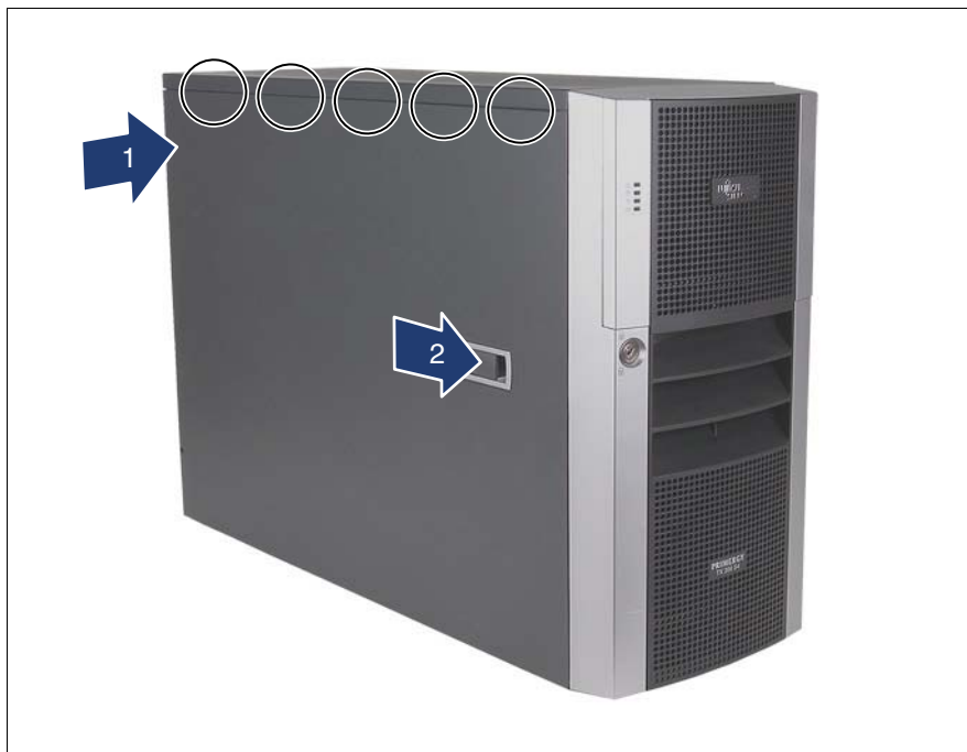
Figure 41: Closing the housing (example: floorstand model)
