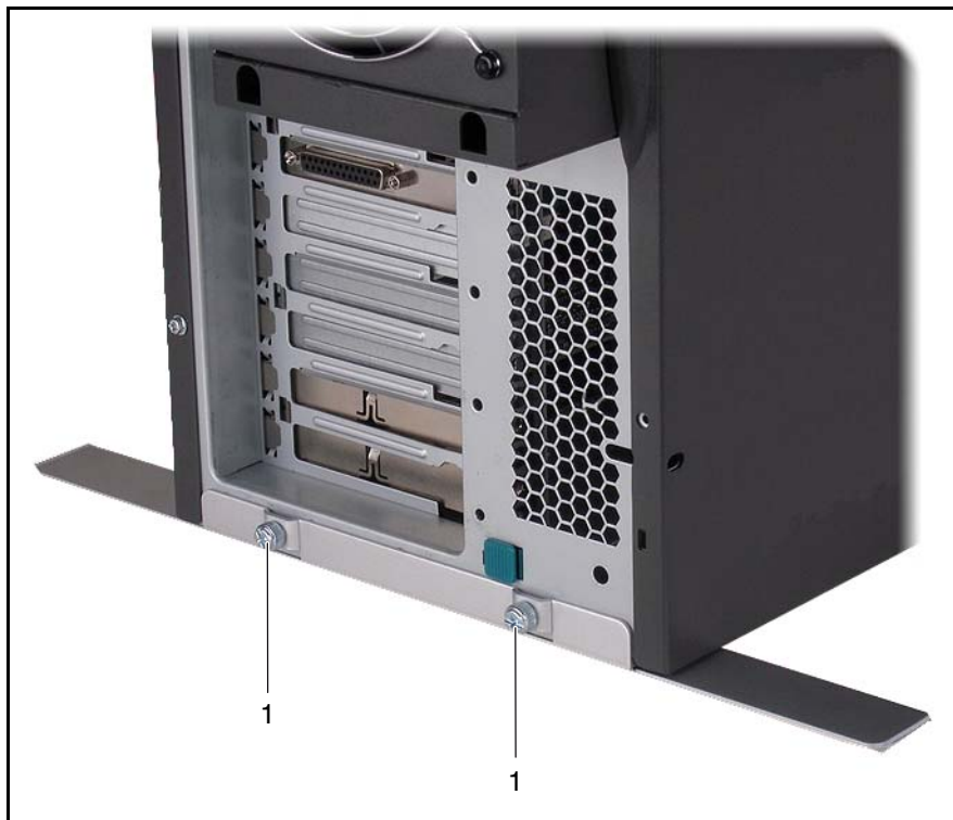
Figure 2: Mounting the anti-tilt bracket
