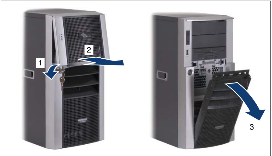
Figure 23: Removing the drive cover and the hard disk cover
