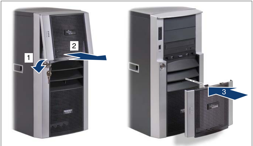
Figure 12: Removing the drive cover and snapping it into the hard disk drive cover
