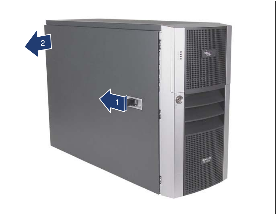
Figure 28: Opening the housing (example: floorstand model)
