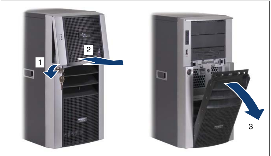
Figure 14: Removing the drive cover and the hard disk cover
