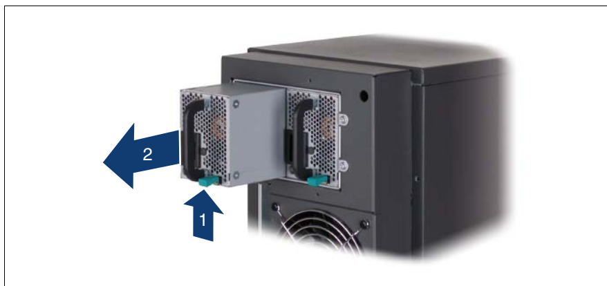
Figure 20: Unlocking and removing the power supply unit
