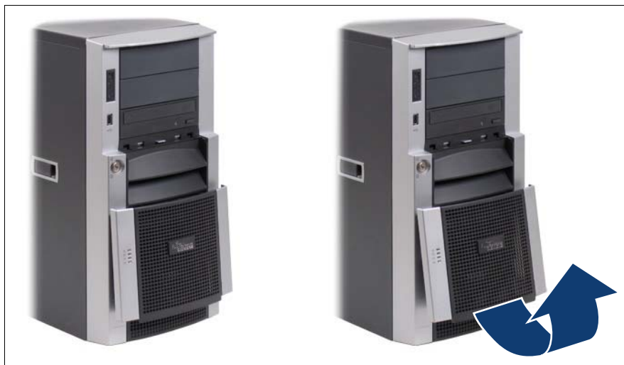
Figure 13: Removing the drive cover from the hard disk drive cover
