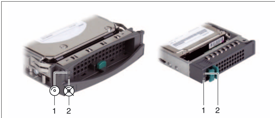
Figure 16: Indicators on the 3.5 inch and 2.5 inch HDD modules
