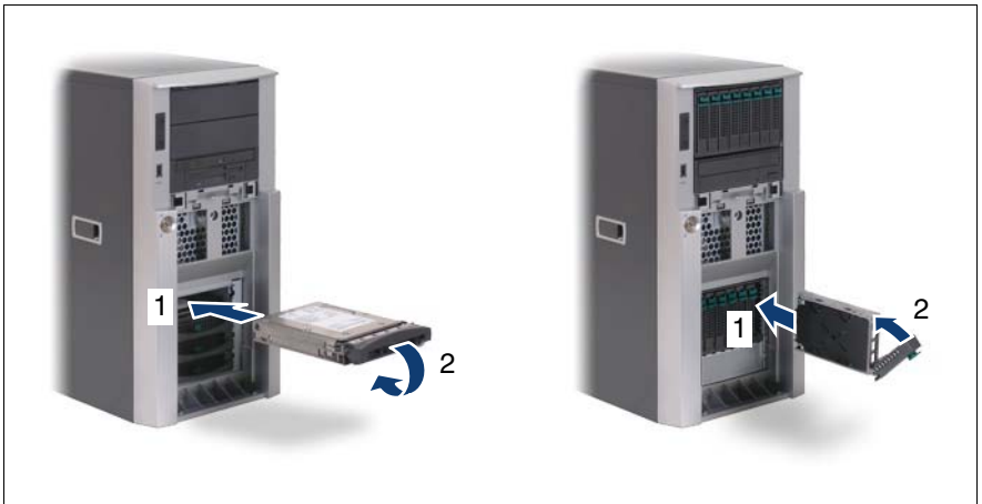
Figure 27: Installing the 3.5-inch and 2.5-inch HDD modules
