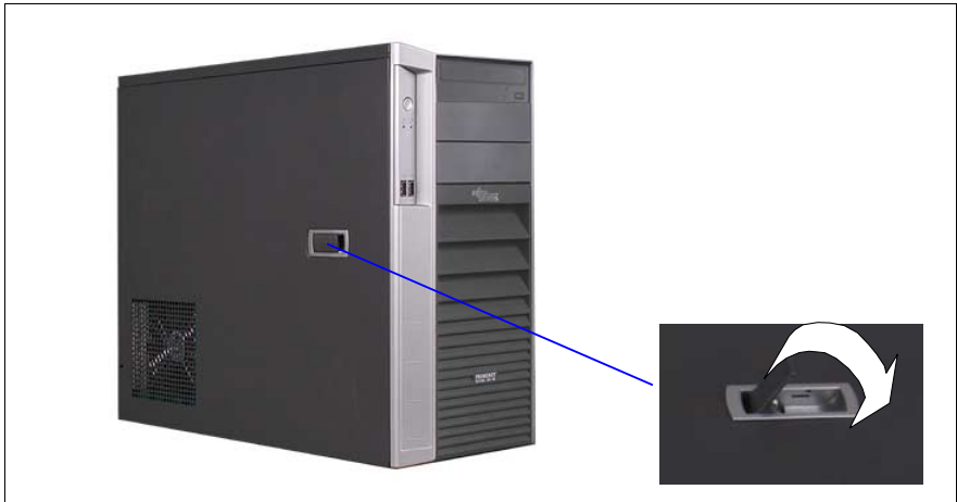
Figure 32: Fastening the side cover
