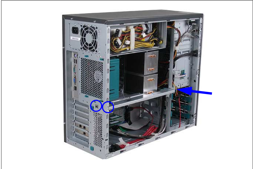
Figure 28: Installing the traverse with the memory air duct
