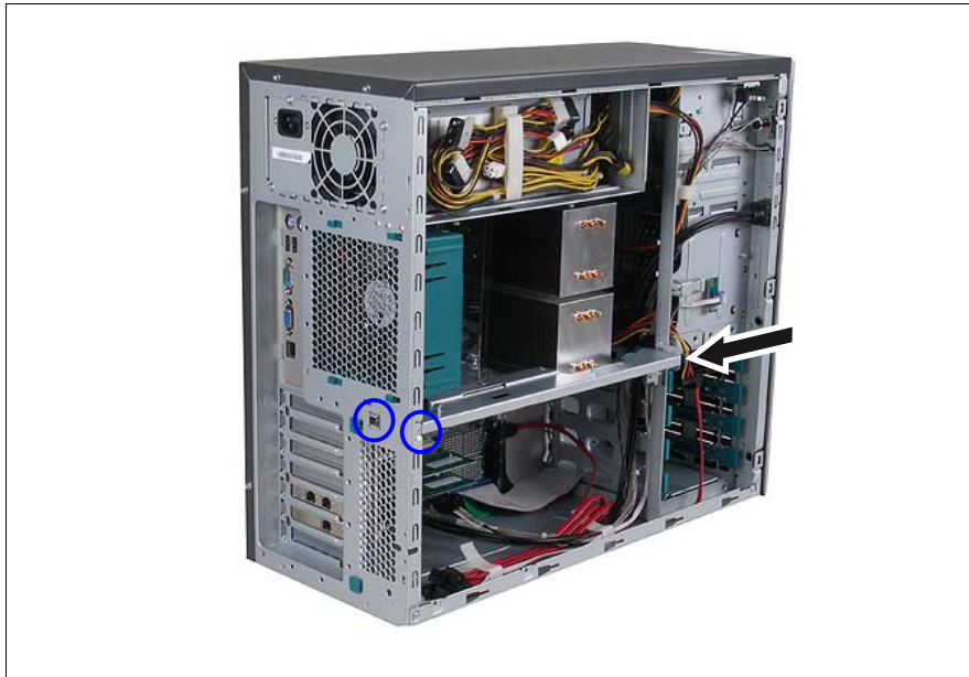
Figure 7: Removing the traverse with the memory air duct
