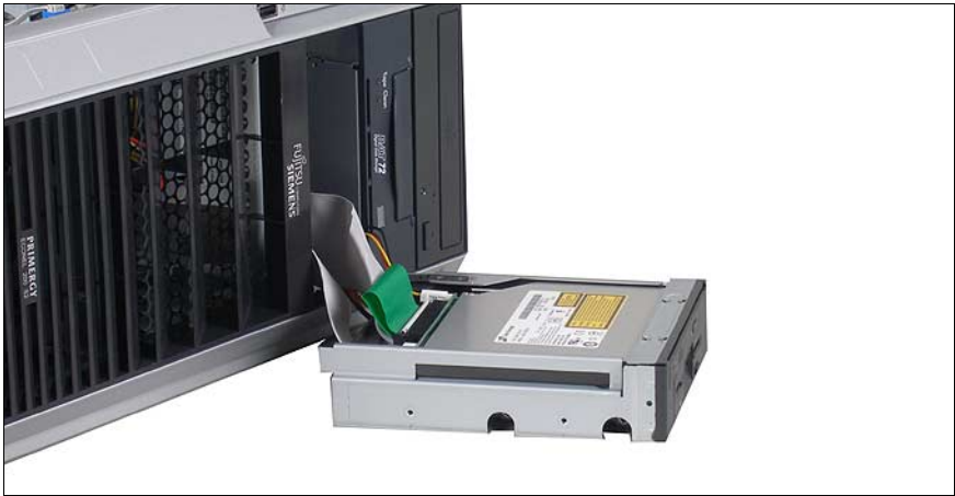
Figure 21: Connecting the cables
