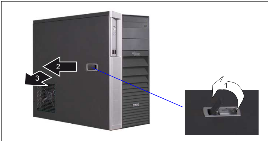
Figure 2: Removing the side cover
