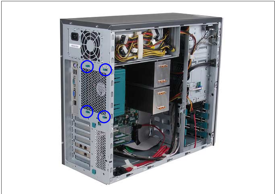
Figure 27: Installing processor fan 1
