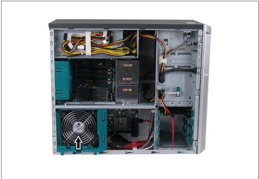
Figure 5: Removing the system fan
