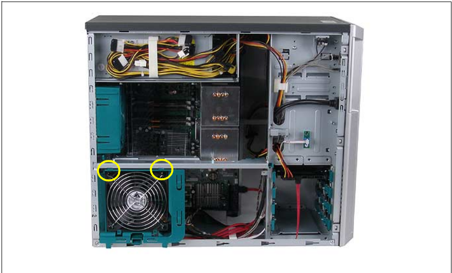
Figure 29: Installing the system fan
