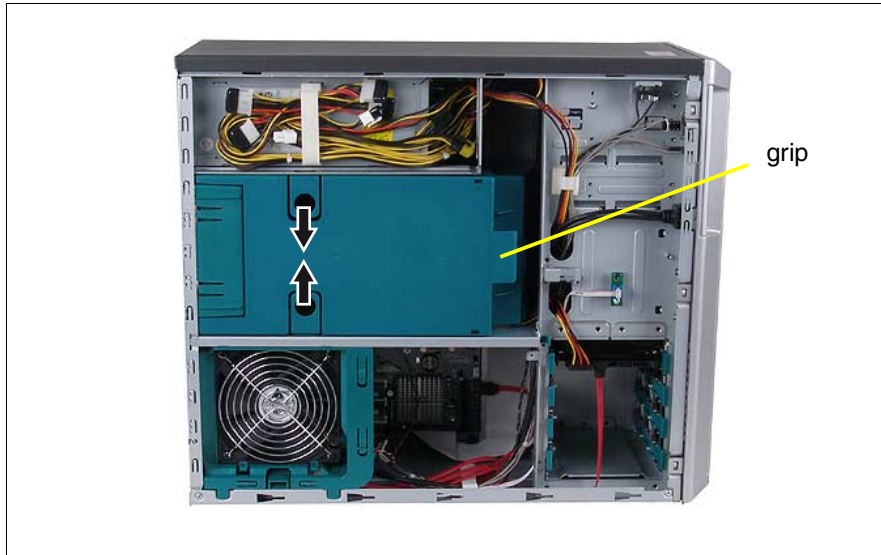
Figure 4: Removing the processor fan 2
