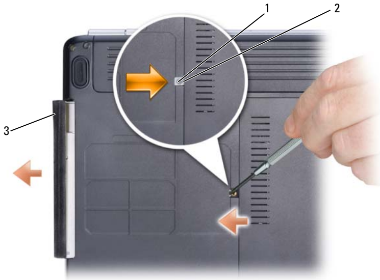
1 locking screw 2 notch 3 optical drive
