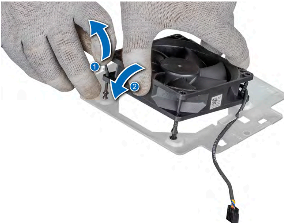
Figure 39. Installing system fan
