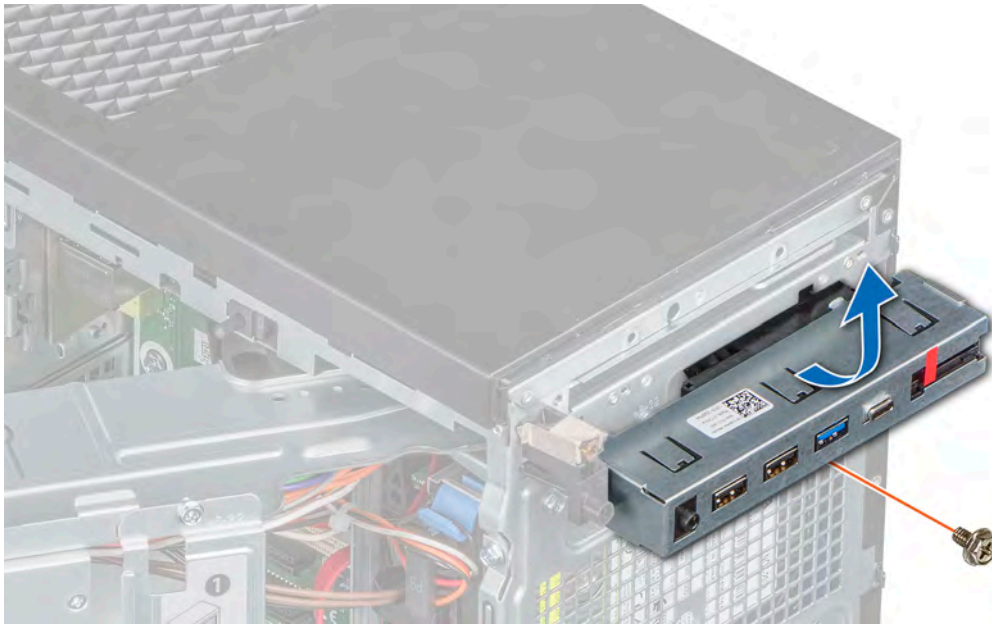
Figure 52. Removal of the control panel
