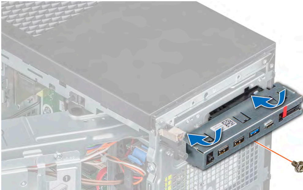
Figure 53. Installing the control panel
