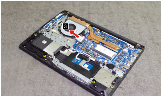
Figure 15. Disconnect the cable and remove the HDD board
