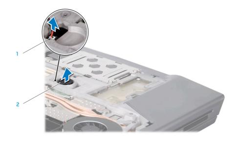
coin-cell battery cable connector 2 coin-cell battery
