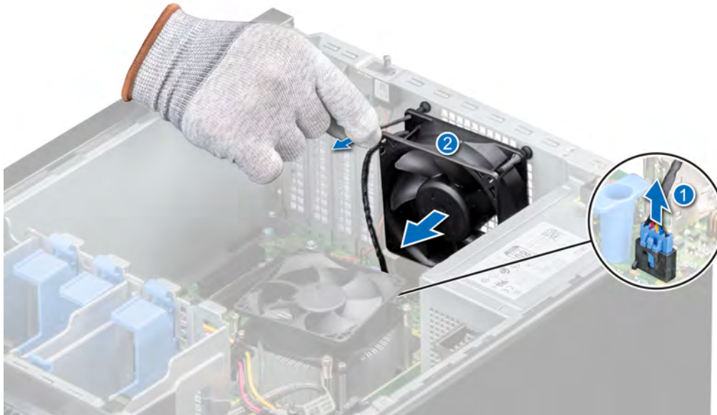
Figure 26. Removing the cooling fan
