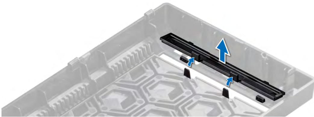
Figure 17. Removing the optical drive filler from the front bezel
