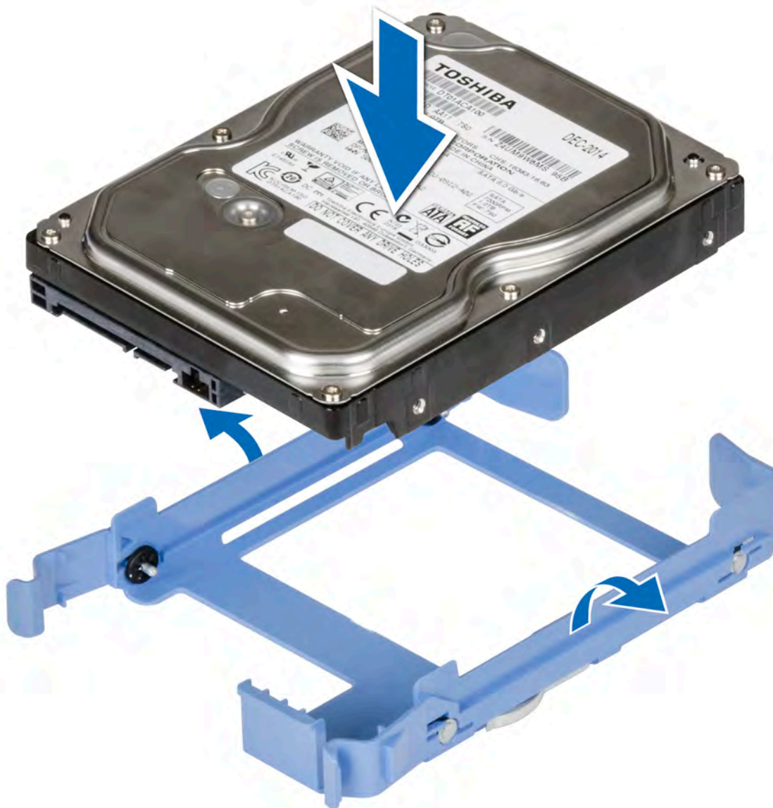
Figure 16. Installing a drive into the drive carrier
