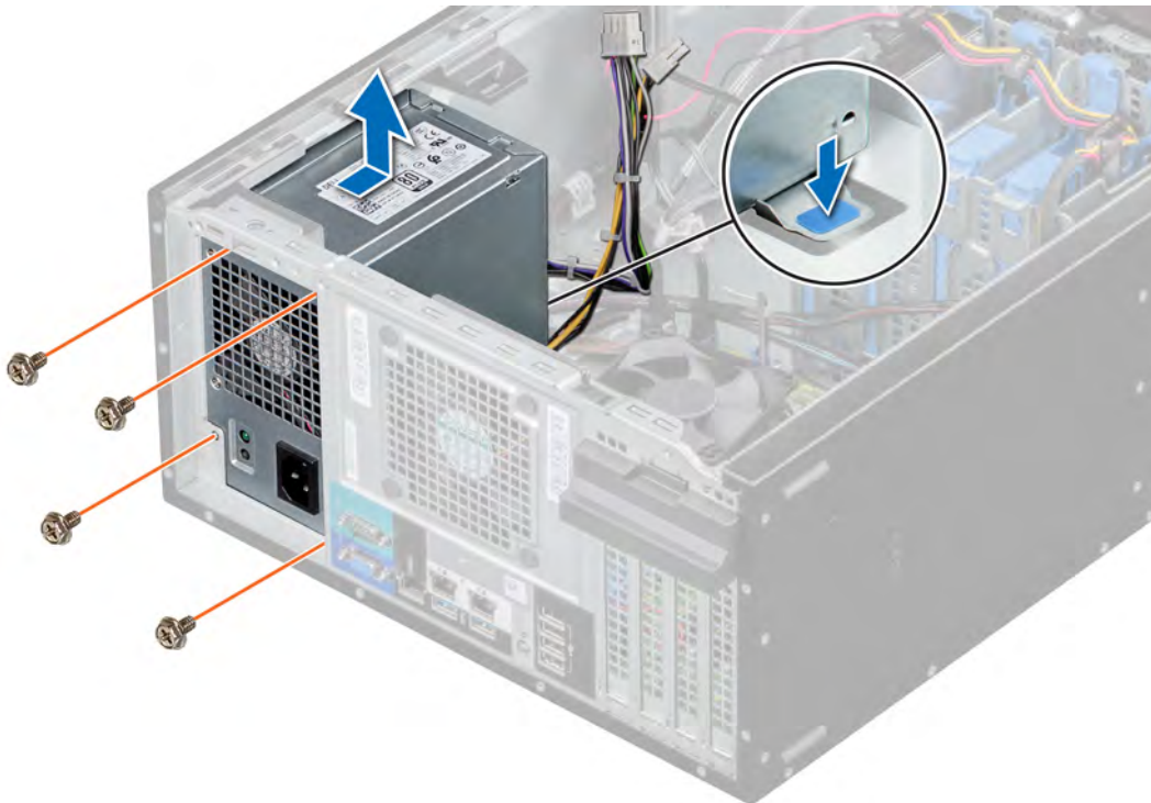
Figure 43. Removing the PSU
