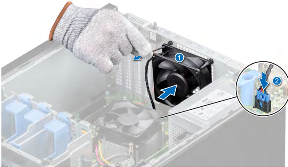
Figure 27. Installing a cooling fan
