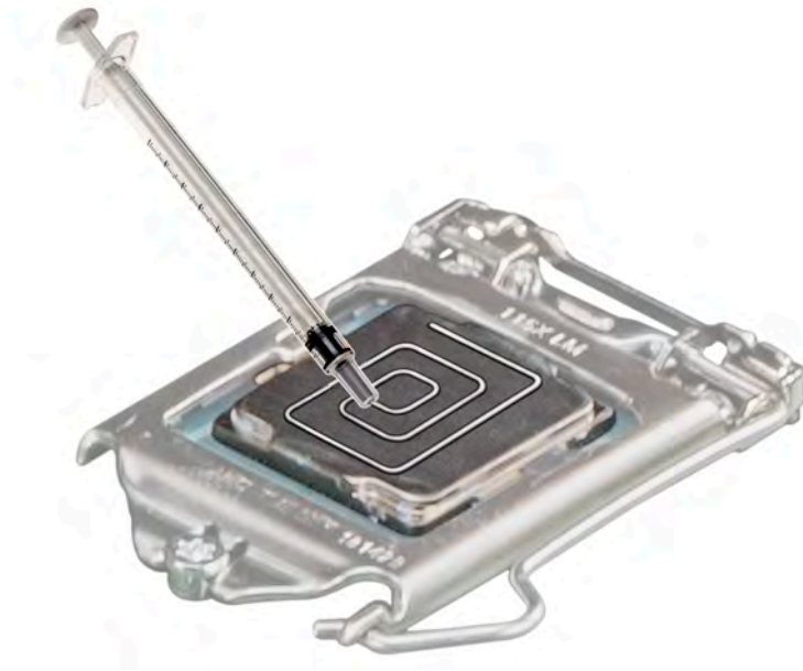
Figure 41. Applying thermal grease on top of the processor
