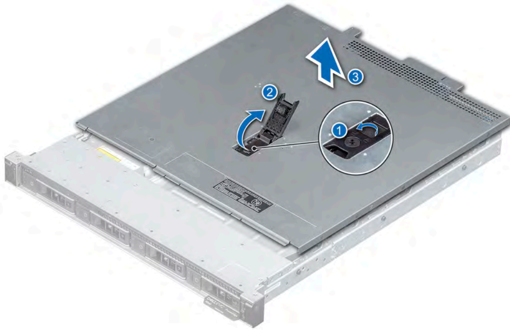
Figure 15. Removing the system cover
