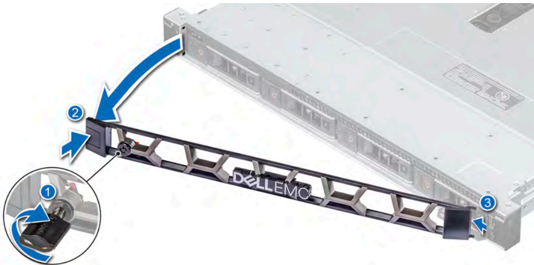
Figure 13. Removing the optional front bezel
