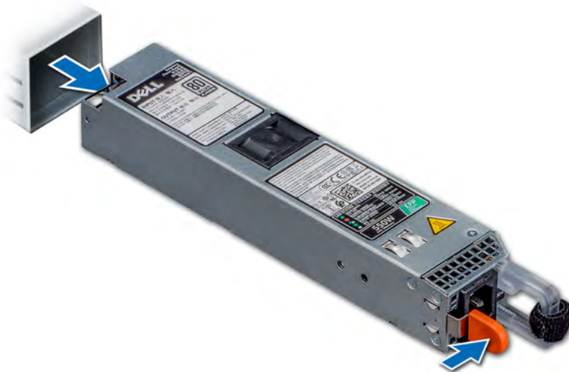
Figure 70. Removing a power supply unit
