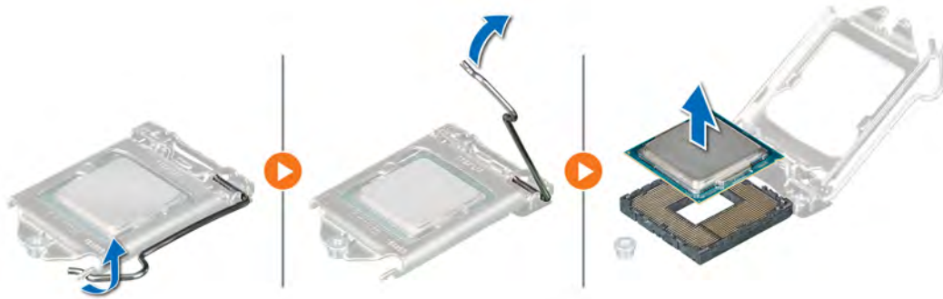
Figure 52. Removing the processor
