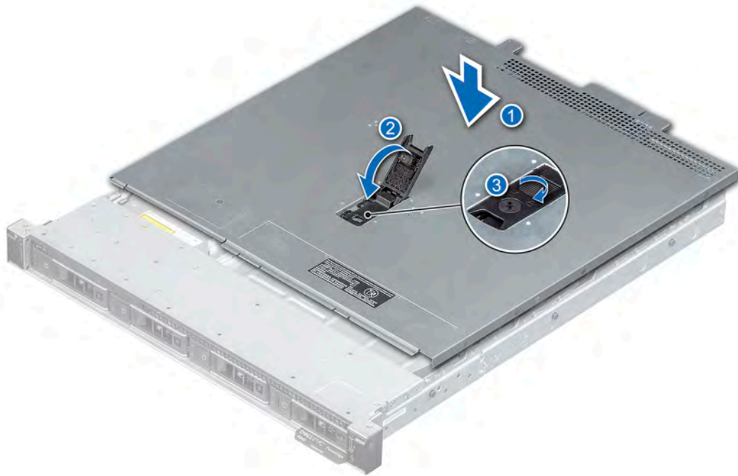
Figure 16. Installing the system cover
