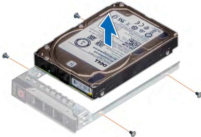
Figure 27. Removing the drive from the drive carrier
