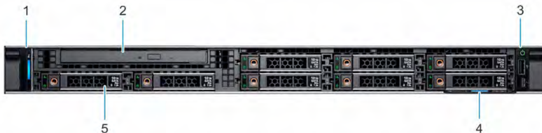
Figure 1. Front view of the 8 x 2.5-inch drive system
