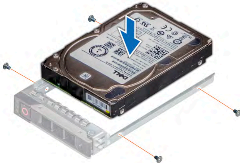
Figure 28. Installing a drive into the drive carrier
