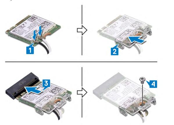
**5** Route the antenna cables on to the securing clips on the system board.
