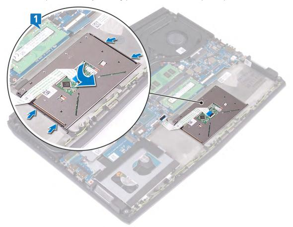
Replace the four screws (M2x2.5) that secure the touchpad to the palm-rest assembly.
