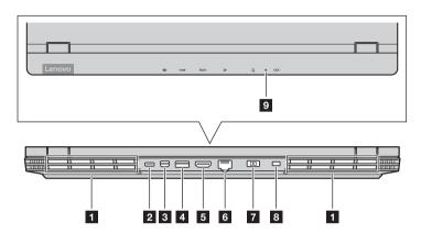
**Ventilation slots** Dissipate internal heat.
