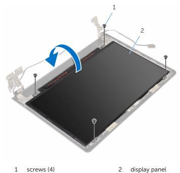
**3** Peel off the tape that secures the display cable to the display panel.
