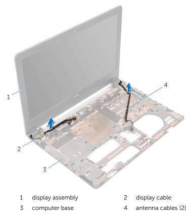
8 Remove the screws that secure the display hinges to the computer base.
