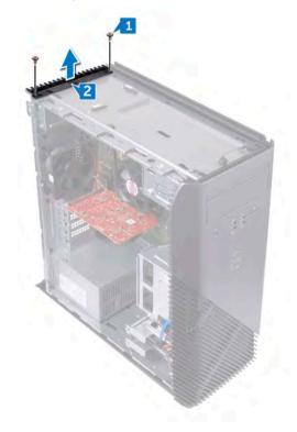
3 Place the computer with the left side-chassis facing up and release the slots on the rear cover from the tabs on the chassis and remove the rear cover from the chassis.
