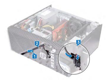
4 Route the cables through the routing guides on the chassis and connect the front panel light-board cable to the system board.
