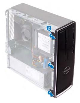
3 Rotate and pull the front bezel away from the computer to release the tabs on the front bezel from the front-panel slots.
