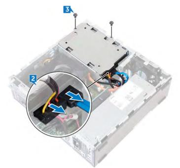
4 Slide the hard-drive assembly toward the inside of the computer and lift it off the drive cage.
