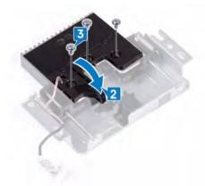
4 Press the top of the retractable-camera assembly to retract the retractable camera.
