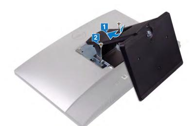
3 Snap the tabs on the stand cover into the slots on the back cover.
