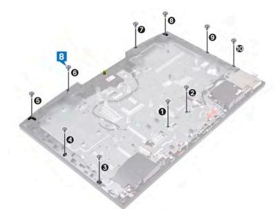
9 Remove the jig screw from the display panel.
