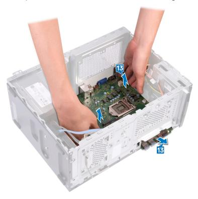
14 Lift the system board and remove it from the chassis.
