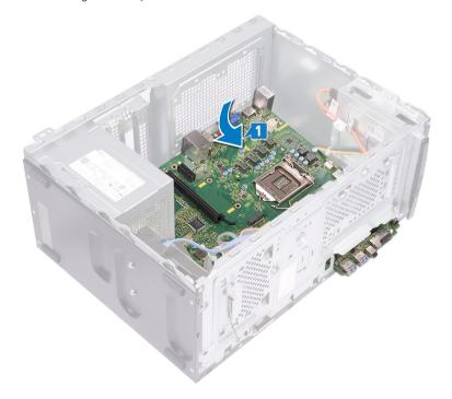
2 Align the screw holes on the system board with the screw holes on the on the chassis.
