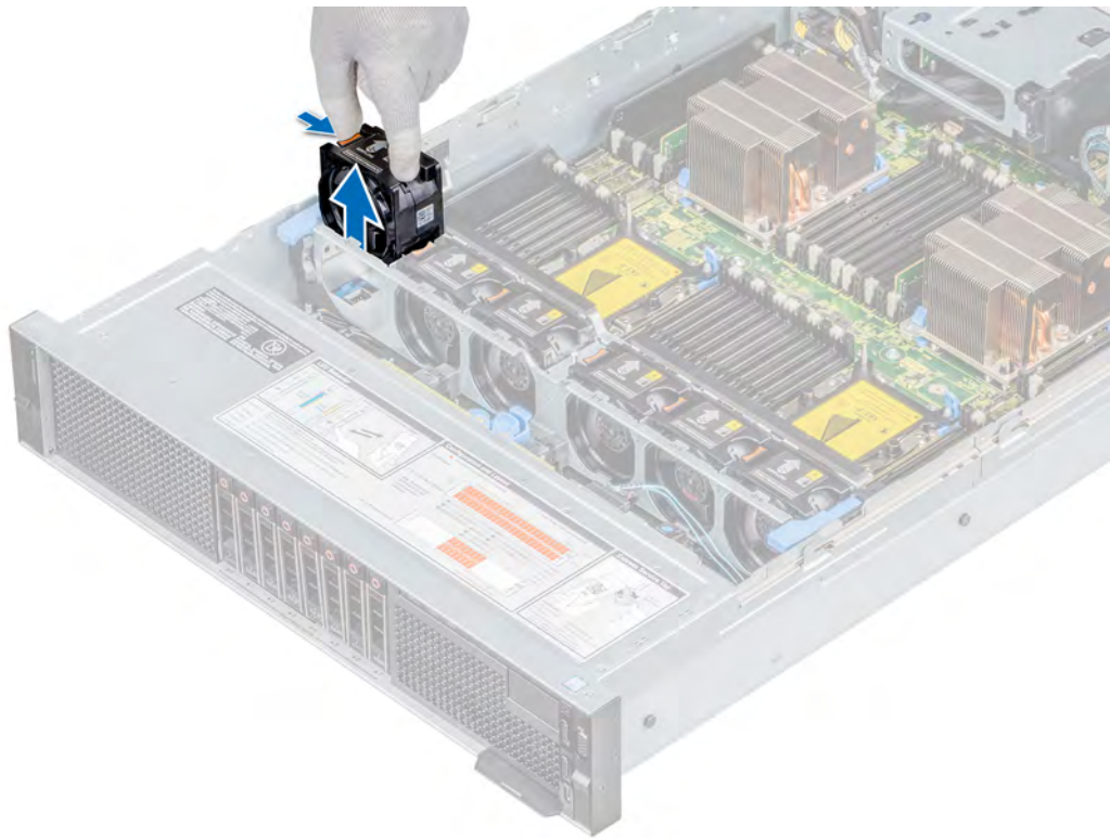
Figure 23. Removing cooling fan
