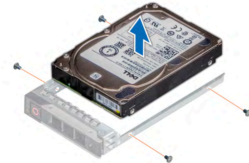
Figure 33. Removing the drive from the drive carrier
