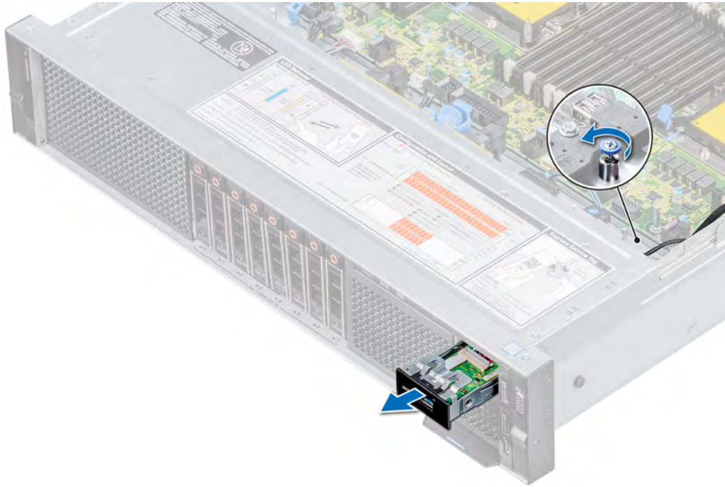
Figure 94. Removing USB 3.0 module
