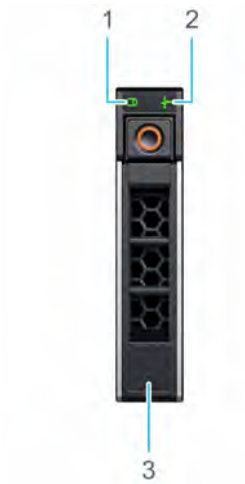
Figure 118. Drive indicators on the drive and the mid drive tray backplane
