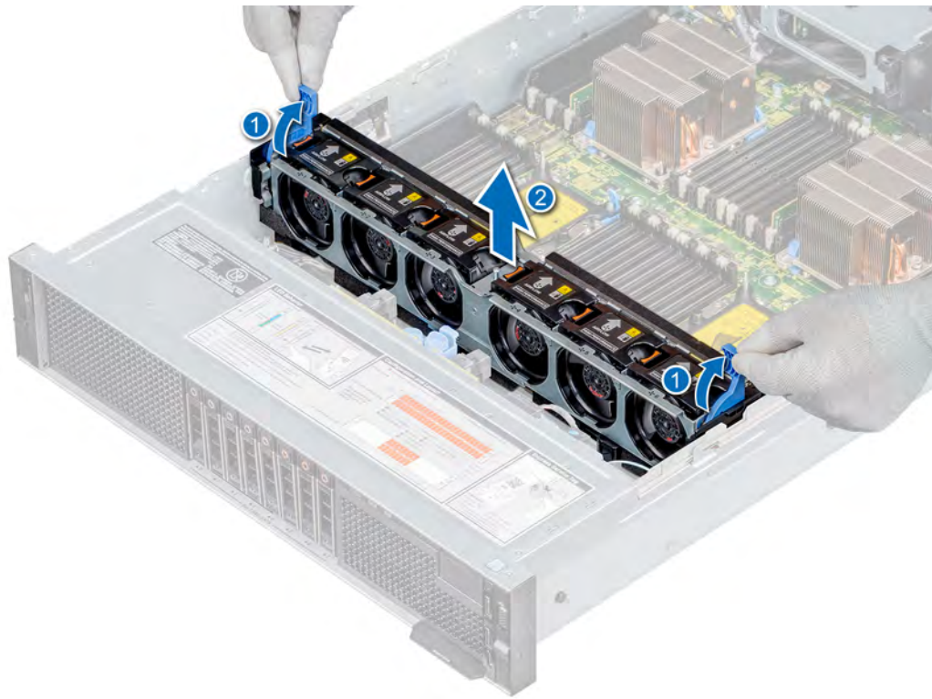
Figure 21. Removing the cooling fan assembly
