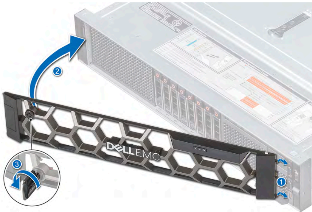
Figure 12. Installing the optional front bezel
