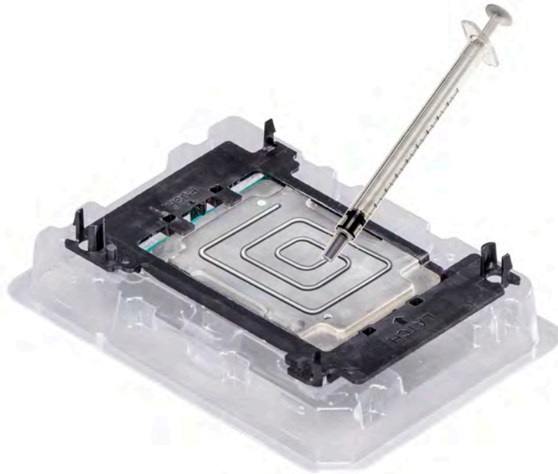
Figure 65. Applying thermal grease on top of the processor
