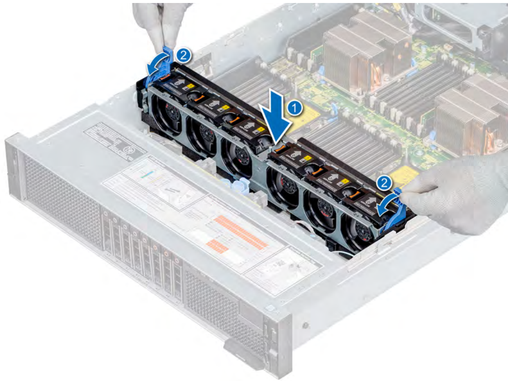
Figure 22. Installing the cooling fan assembly
