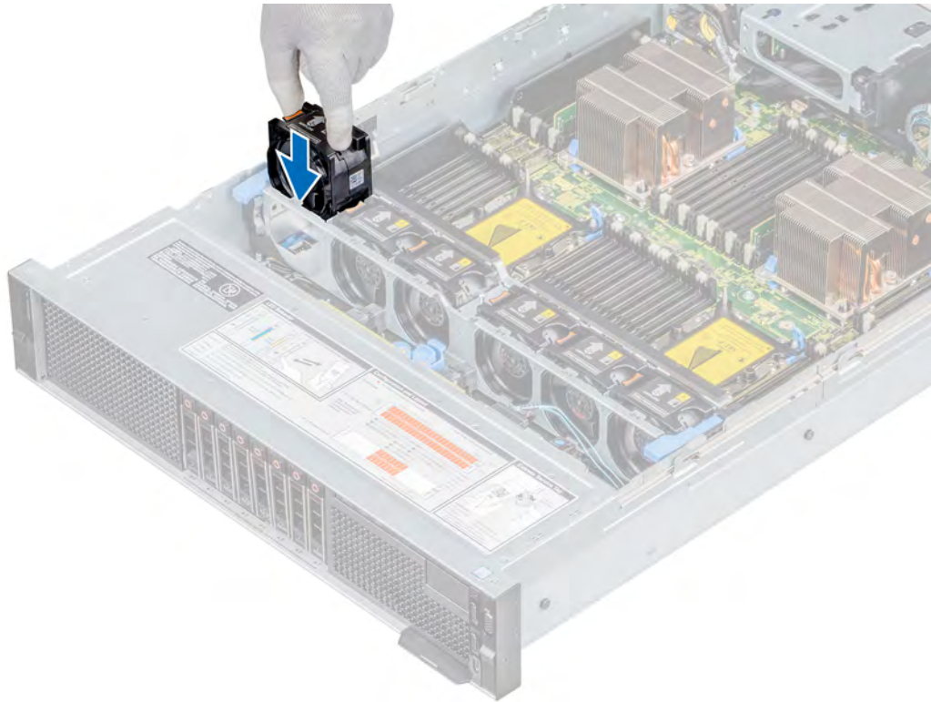
Figure 24. Installing cooling fan
