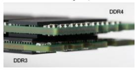
Figure 2. Thickness difference
