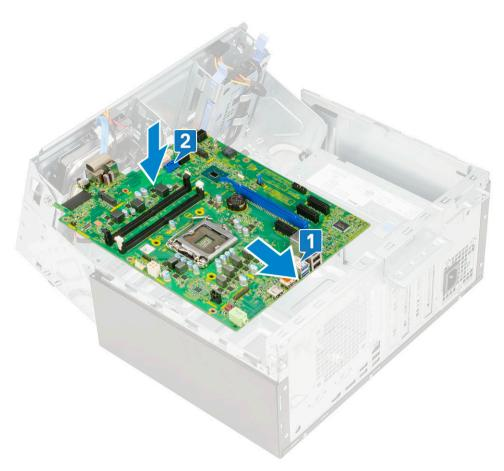
Replace the screws to secure the system board to the computer [1].
