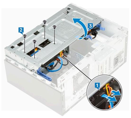
c Remove the 3.5 inch hard drive out of the system.
