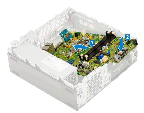
3 Replace the single (#6-32) screw, single (M3x5) screw and 5 screws that secure the system board to the system [1,2].
