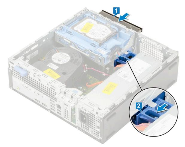
3 Lift the hard drive and optical module [1], connect the optical drive data cable and power cable to the connectors on the optical drive [2, 3].
