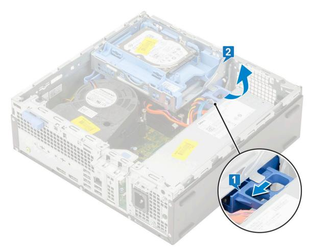
d Disconnect the optical drive data cable and optical drive power cable from the connectors on the optical drive [1, 2] and lower the hard drive and optical module until it is seated.
