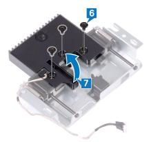
Pull the clip on the retractable-camera assembly, and rotate the camera and camera bracket along with the camera cable, off the retractable-camera assembly.
