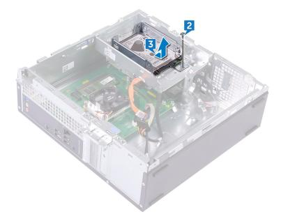
Remove the four screws (M3xL3.5) that secure the hard drive to the hard-drive bracket.
