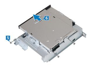
Gently pull and remove the optical-drive bezel from the optical drive.
