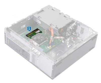
2 Using your fingertips, carefully spread apart the securing clip at each end of the memory-module slot until the memory module pops up.
