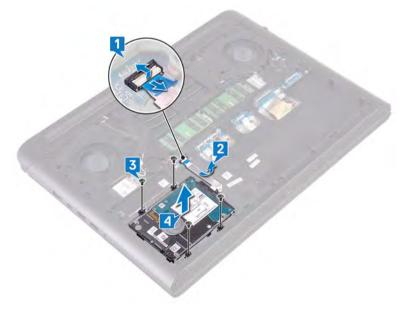
Disconnect the interposer from the hard-drive assembly.
