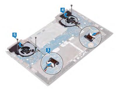
6 Lift the left and right fans off the heat sink.
