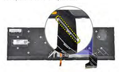
2 Gently fold the keyboard cable with the end aligned at the fold line as shown in the image. Once folded correctly, the right edge of the keyboard cable should be lined up next to the line indicated on the palm-rest assembly.
