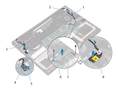
Figure 29. Disconnecting the cables
