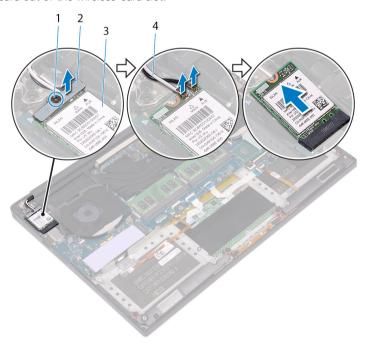
Figure 16. Removing the wireless card
