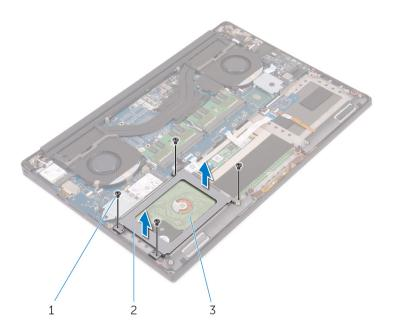
Figure 7. Removing the hard-drive cage
