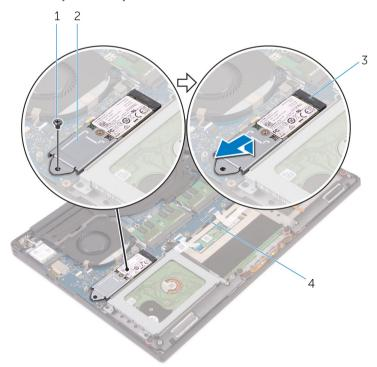
Figure 11. Removing the solid-state drive assembly
