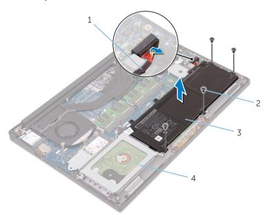
Figure 3. Removing the battery
