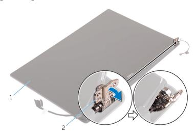
Figure 33. Turning the display hinge
