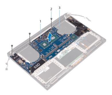
Figure 23. Removing the system board
