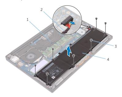
Figure 4. Removing the battery
