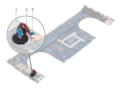
Figure 25. Removing the coin-cell battery
