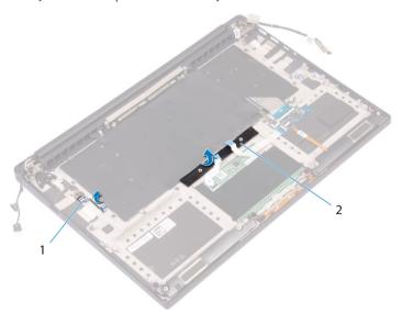
Figure 26. Peeling the Mylar
