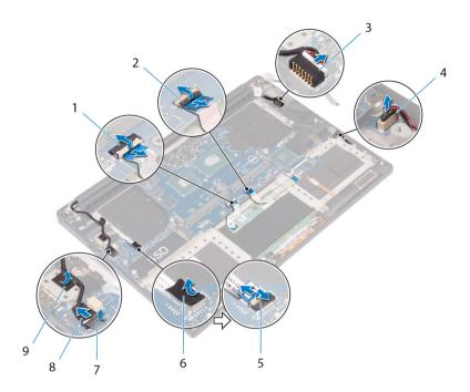
Figure 22. Disconnecting the cables
