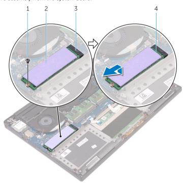
Figure 13. Removing the solid-state drive
