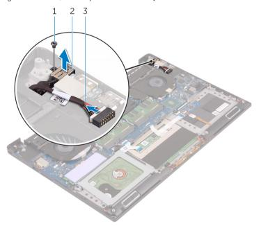
Figure 32. Removing the power-adapter port
