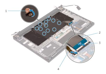
Figure 27. Disconnecting the keyboard and keyboard-backlight cable
