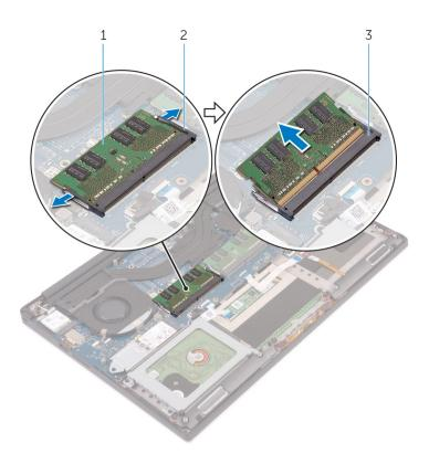
Figure 5. Removing the memory modules
