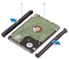
Figure 10. Removing the hard-drive cover
