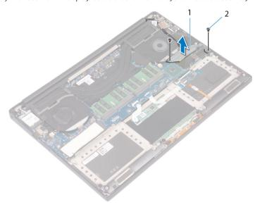
Figure 19. Removing the display-cable bracket
