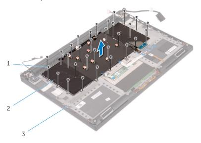
Figure 28. Removing the screws from the keyboard
