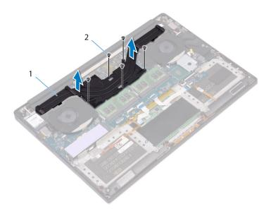
Figure 21. Removing the heat sink
