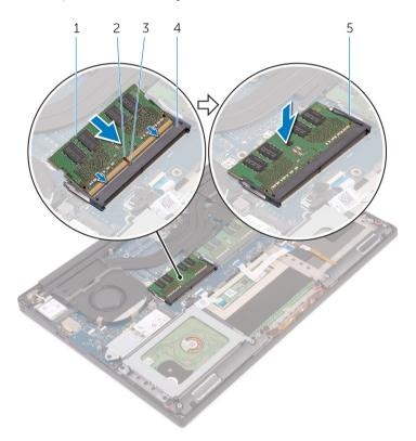
Figure 6. Replacing the memory modules
