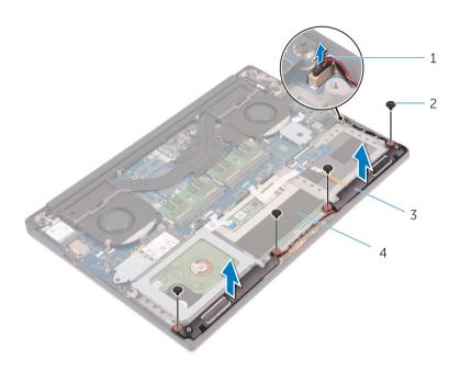
Figure 15. Removing the speakers
