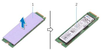
Figure 14. Removing the thermal pad
