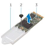
Figure 12. Removing the solid-state drive bracket
