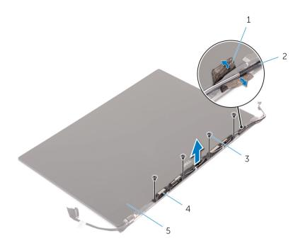
Figure 35. Removing the antenna module
