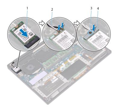
Figure 17. Replacing the wireless card
