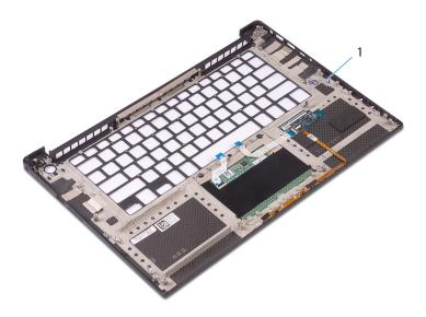
Figure 36. Removing the palm-rest assembly
