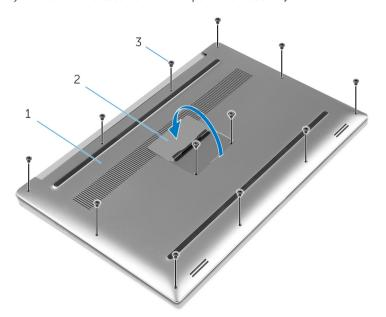
Figure 1. Removing the base cover
