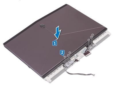
**3** Push the antenna cables through the gap between the display assembly and the system board to reach the other side of the system board.
