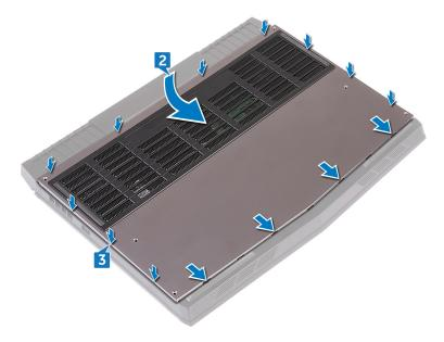
4 Tighten the captive screw that secures the base cover to the computer base.
