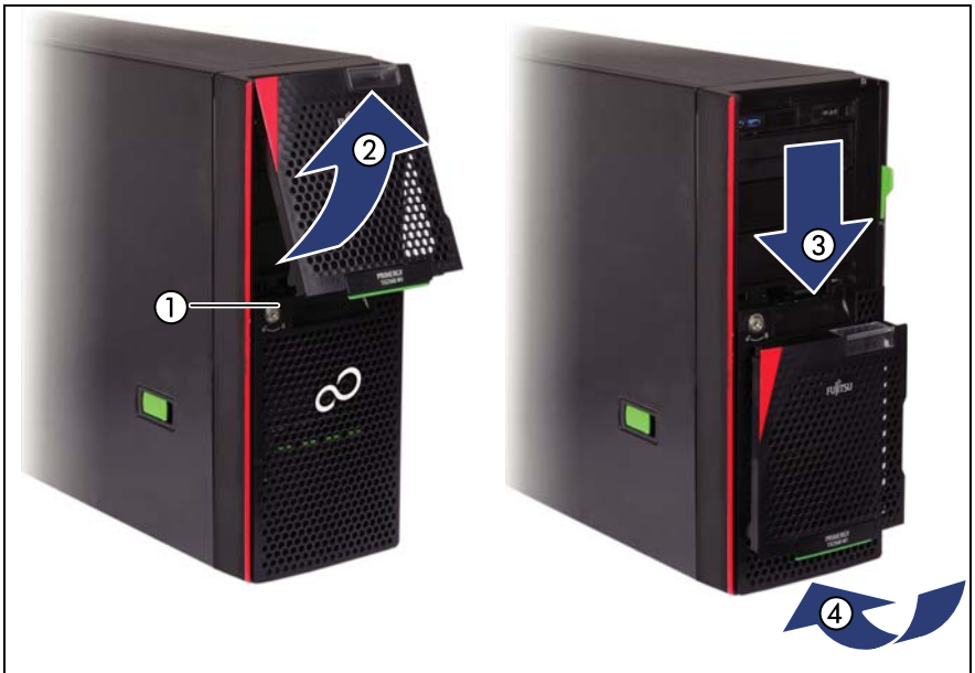
Figure 7: Removing the drive cover and placing it on the HDD cover
