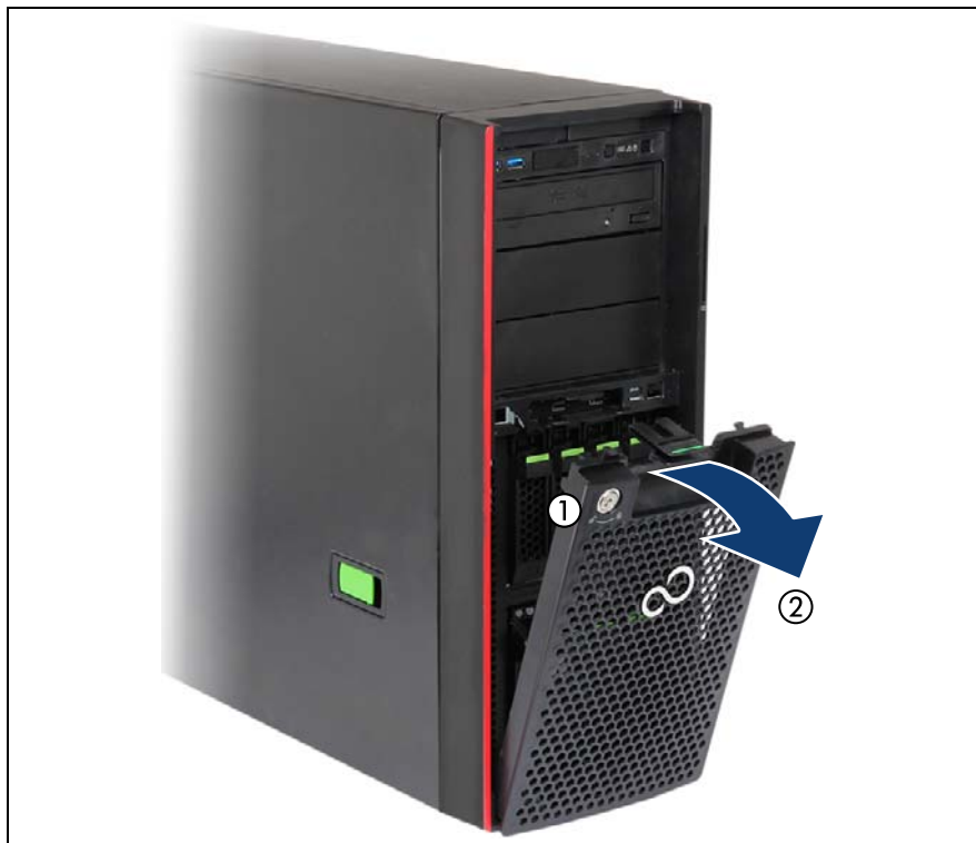
Figure 8: Removing the HDD cover
