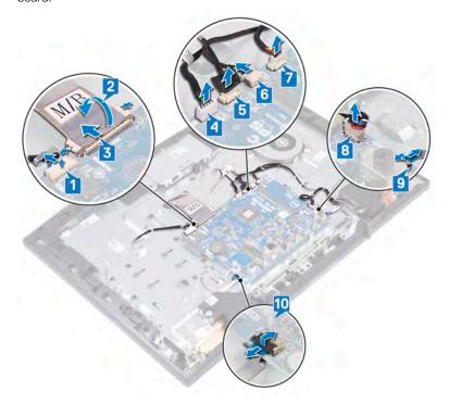
Remove the five screws (M3x5) that secure the system board to the displayassembly base.
