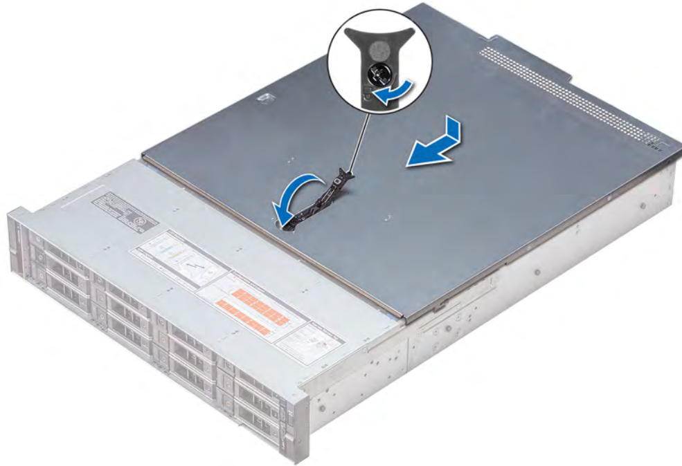
Figure 22. Installing the system cover
