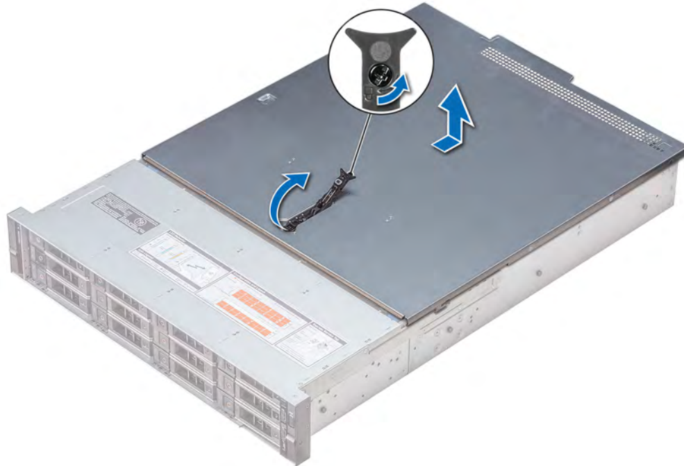
Figure 21. Removing the system cover
