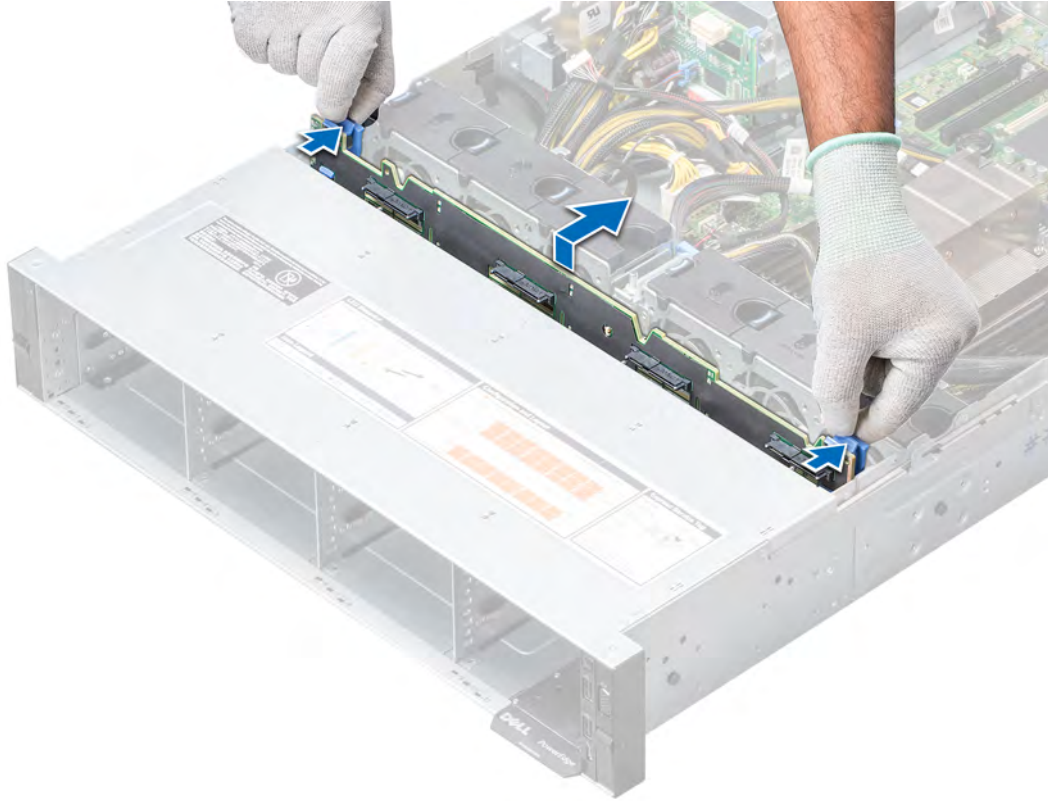
Figure 58. Removing the drive backplane
