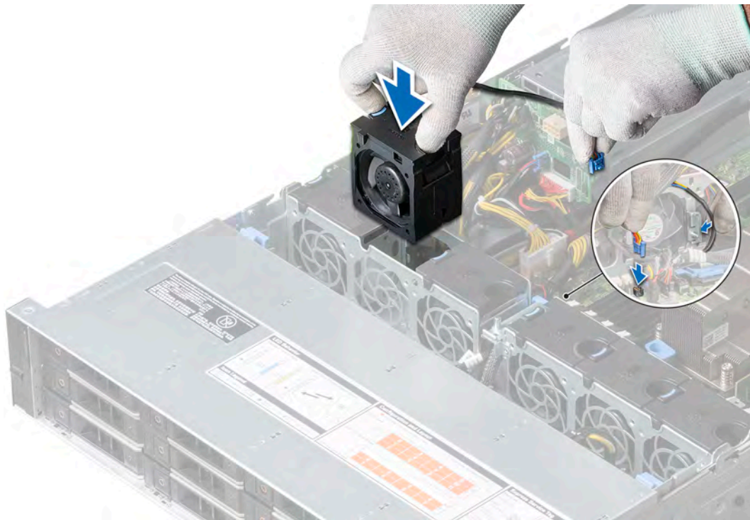
Figure 31. Installing a cooling fan
