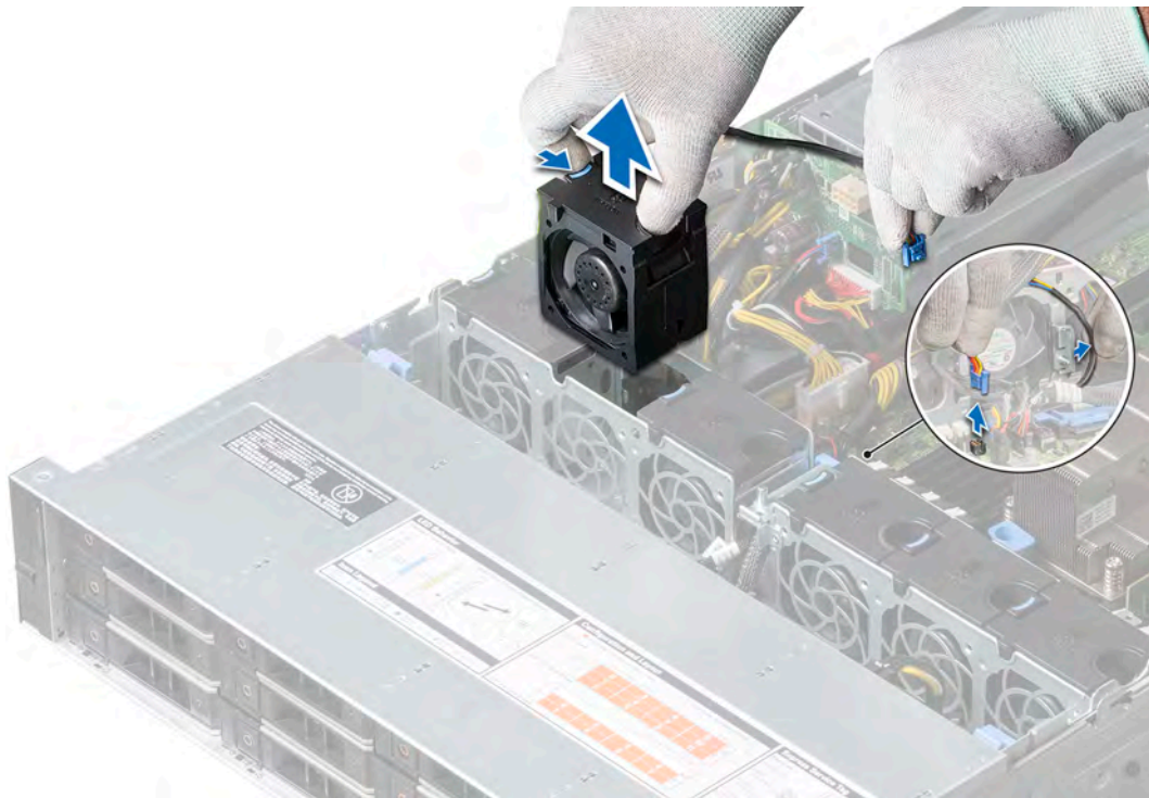
Figure 29. Removing a cooling fan
