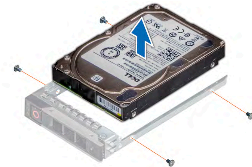
Figure 39. Removing the drive from the drive carrier
