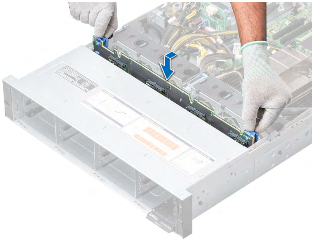
Figure 59. Installing the drive backplane
