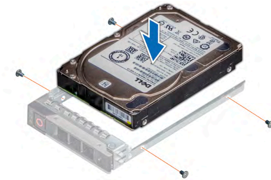
Figure 40. Installing a drive into the drive carrier
