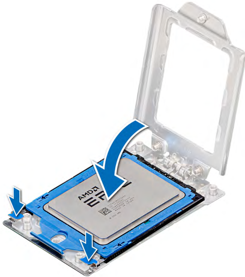
Figure 46. Closing the processor socket frame
