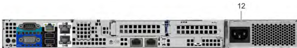
Figure 13. Back view of the system with cabled PSU
