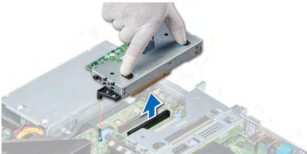
Figure 49. Removing the low profile left riser
