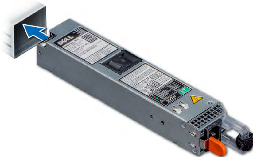
Figure 83. Installing a hot swappable PSU
