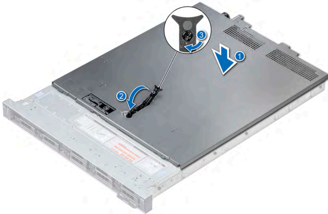
Figure 22. Installing system cover
