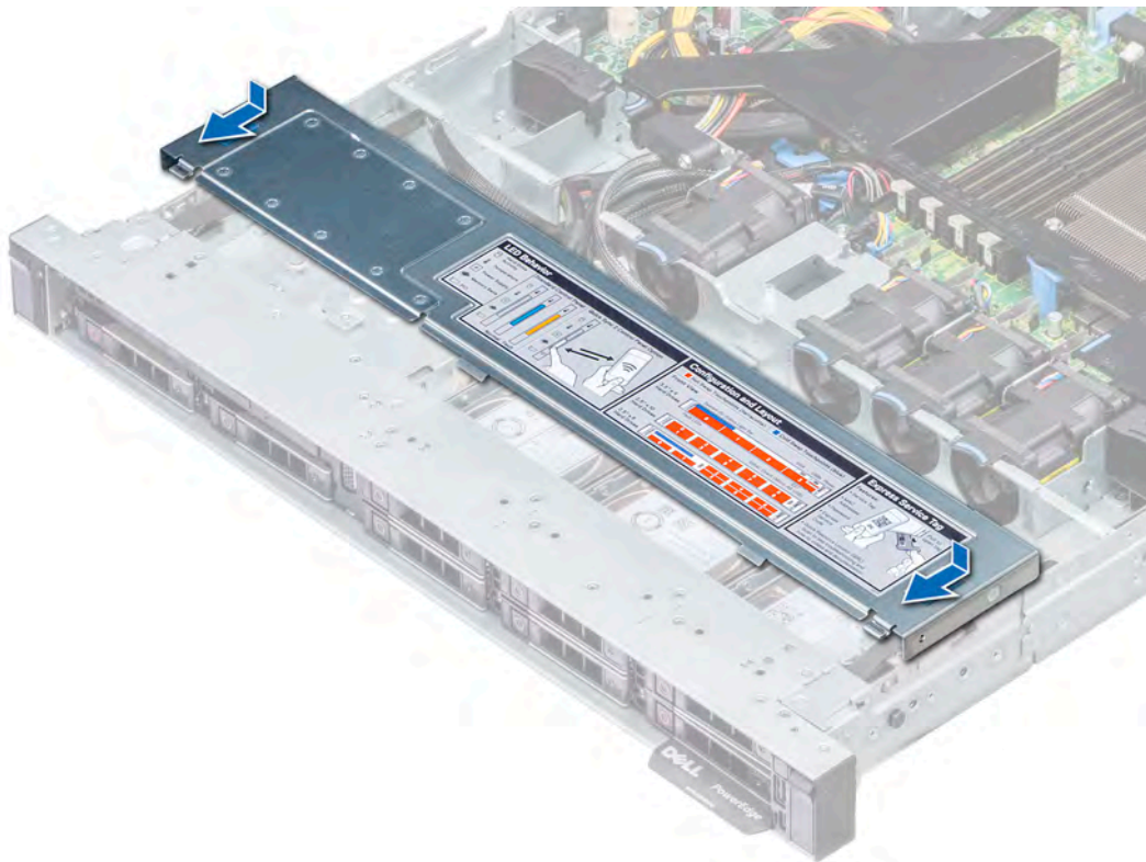
Figure 24. Installing backplane cover
