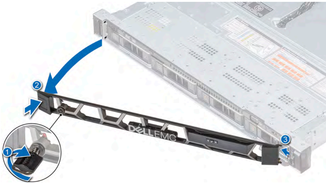
Figure 19. Removing the front bezel with the LCD panel
