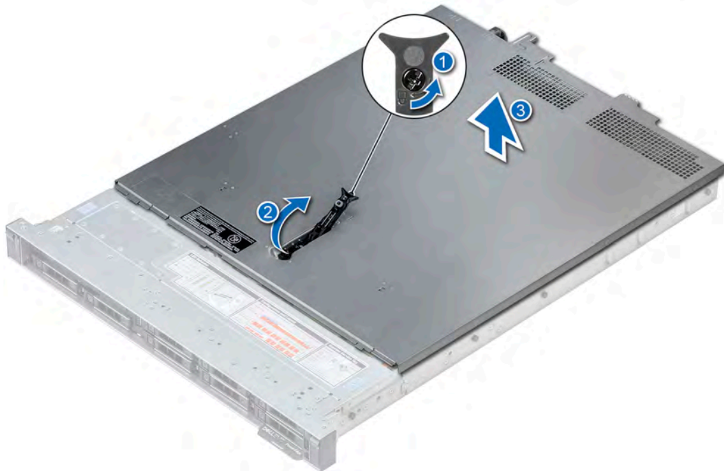
Figure 21. Removing the system cover
