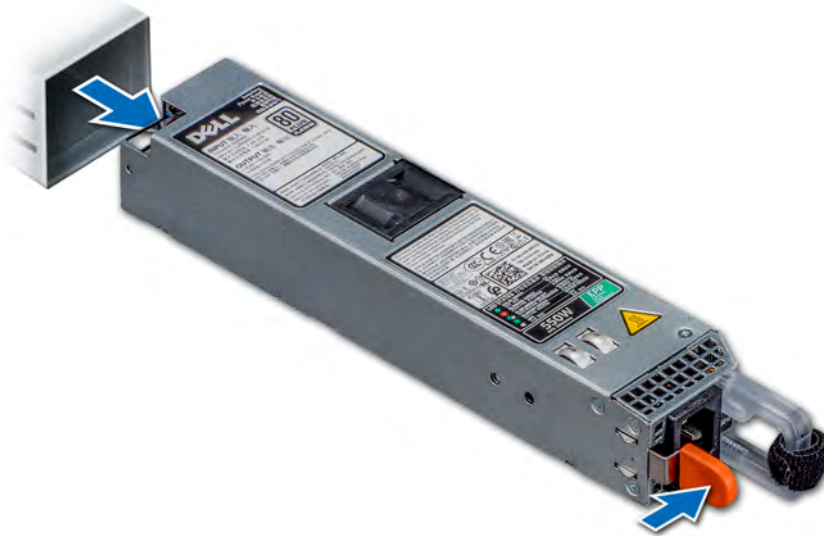
Figure 82. Removing a power supply unit
