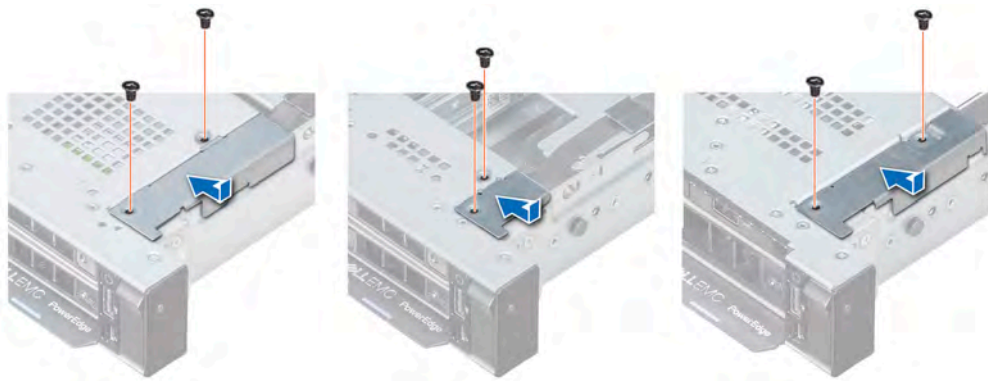
Figure 93. Installing the cable cover
