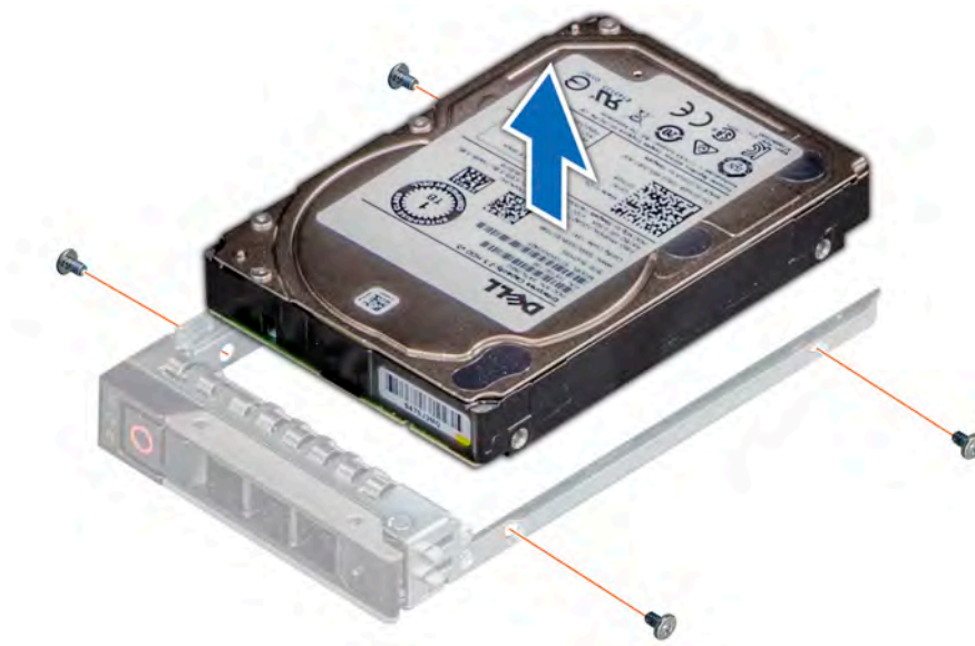
Figure 36. Removing the drive from the drive carrier
