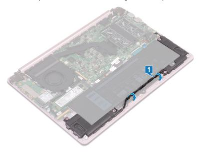
**2** Remove the four screws (M2x3) that secure the battery to the palm-rest and keyboard assembly.
