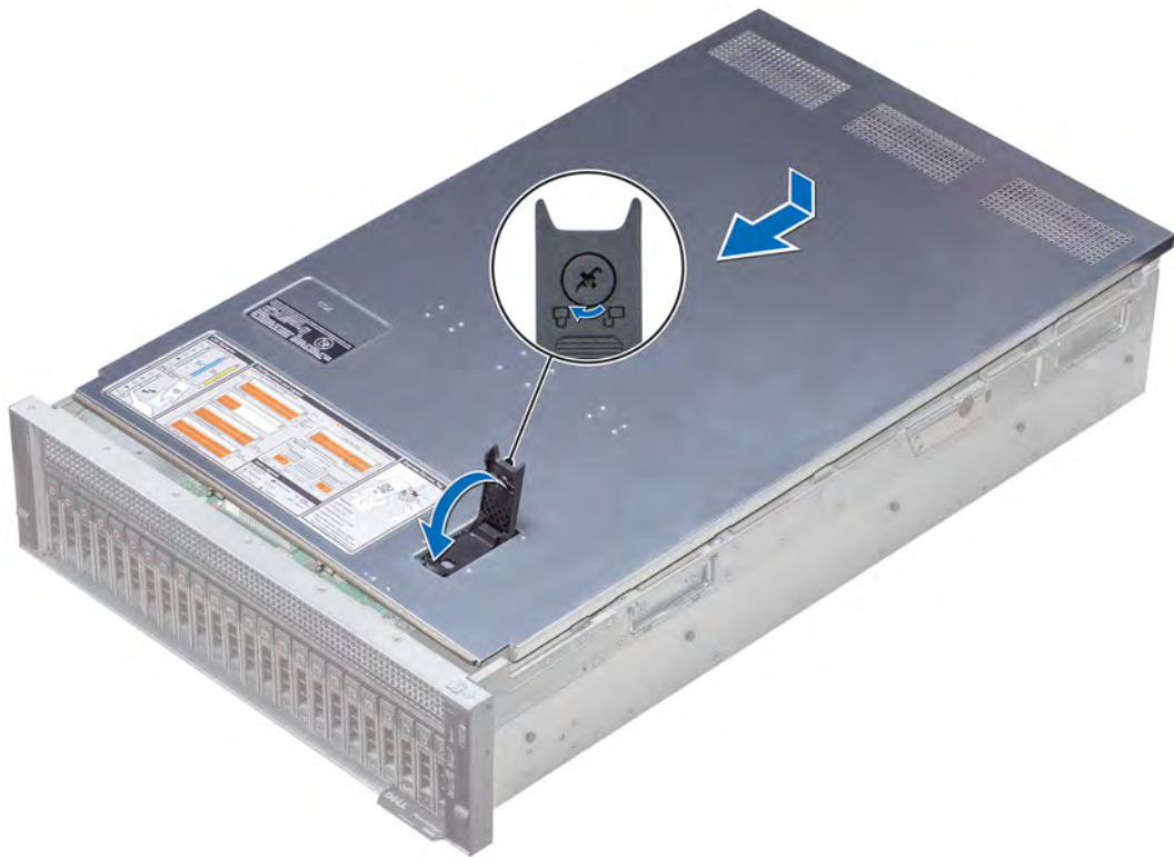
Figure 18. Installing the system cover
