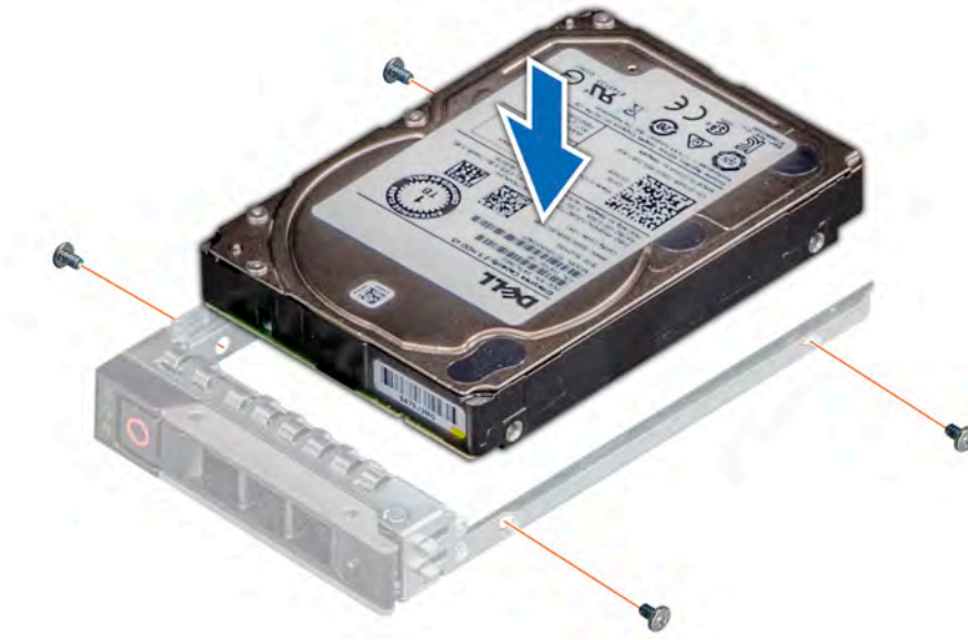
Figure 38. Installing a drive into the drive carrier
