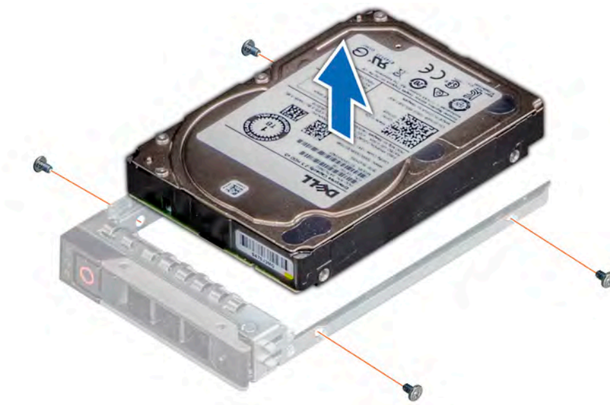
Figure 37. Removing the drive from the drive carrier
