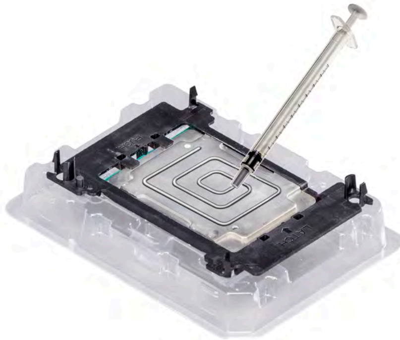
Figure 59. Applying thermal grease on top of the processor
