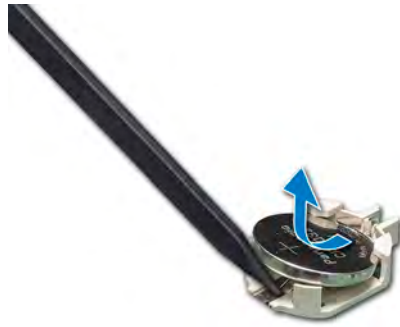
Figure 93. Removing the system battery
