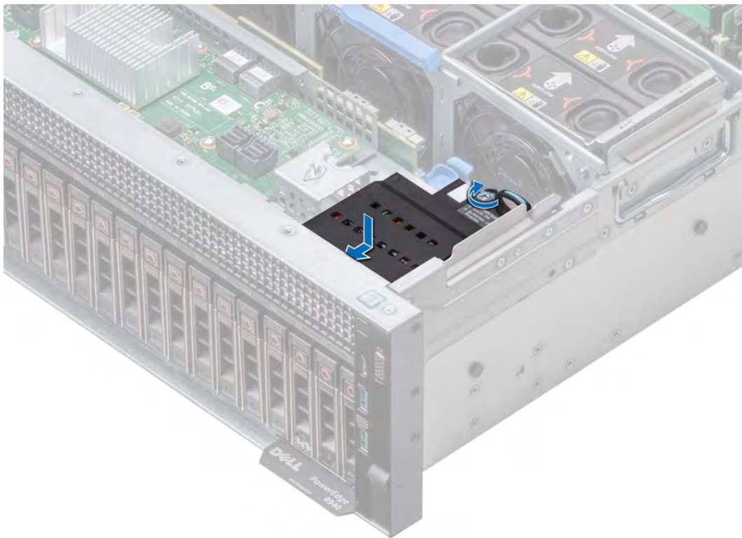
Figure 91. Installing NVDIMM-N battery
