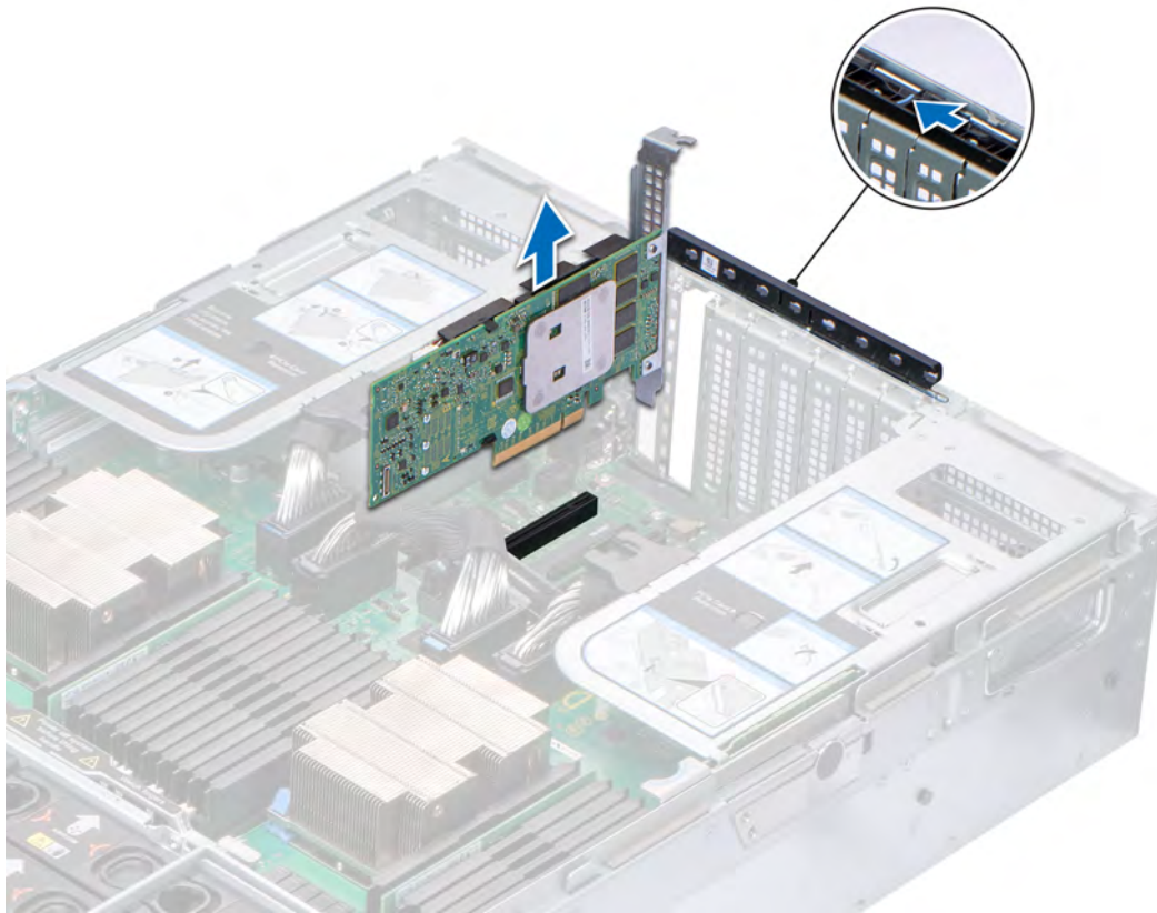
Figure 82. Removing the storage controller card
