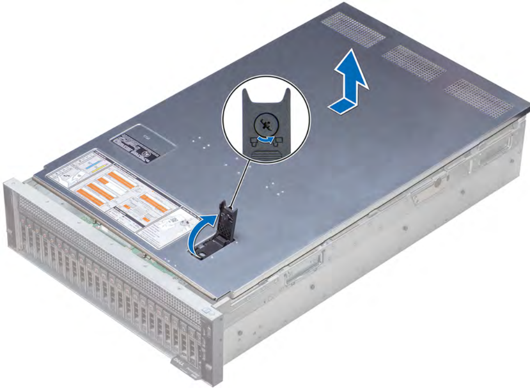
Figure 17. Removing the system cover
