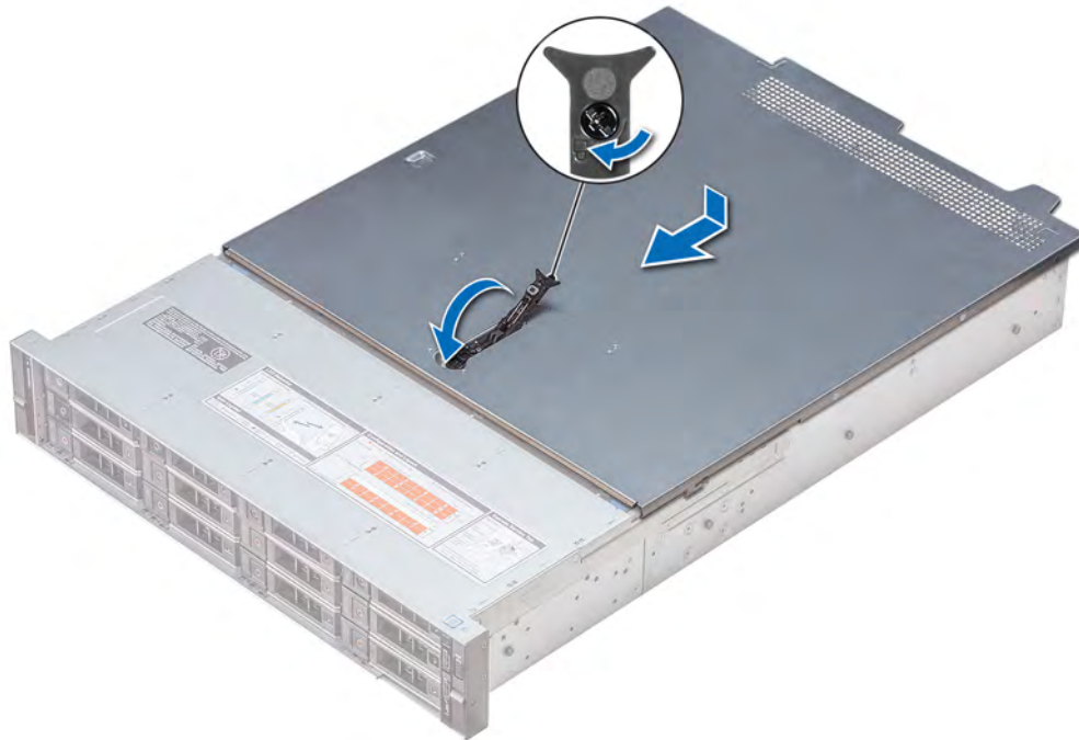
Figure 26. Installing system cover
