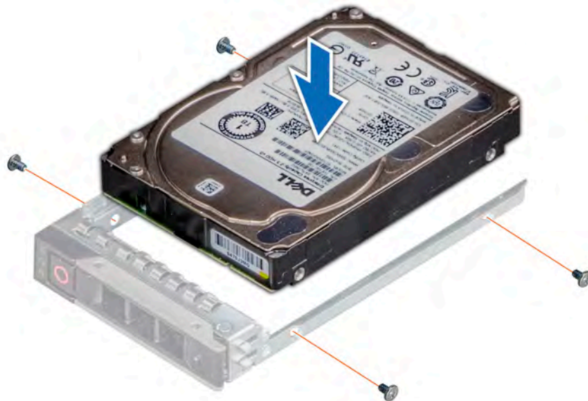
Figure 54. Installing a drive into the drive carrier
