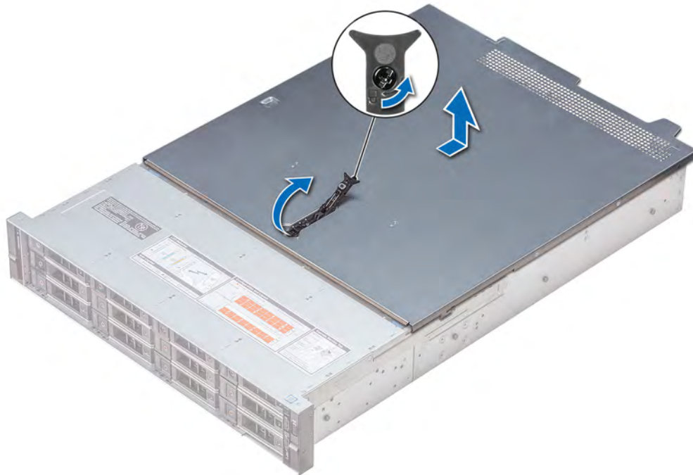
Figure 25. Removing the system cover
