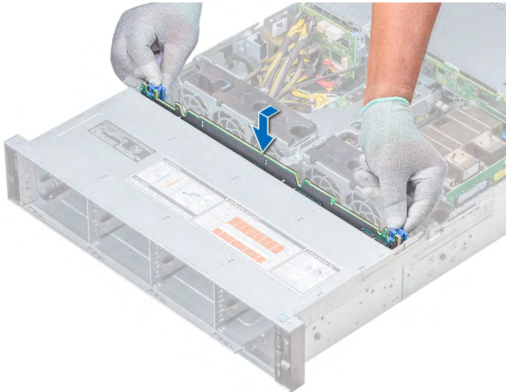
Figure 102. Installing the backplane
