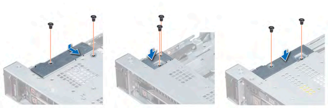
Figure 101. Installing the cable cover
