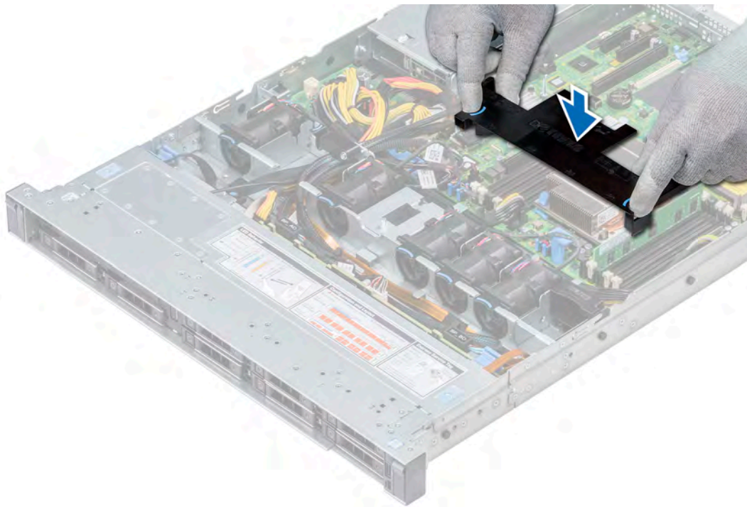
Figure 25. Installing the air shroud
