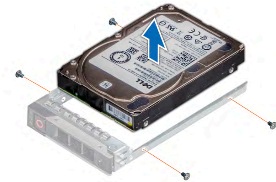
Figure 38. Removing the drive from the drive carrier
