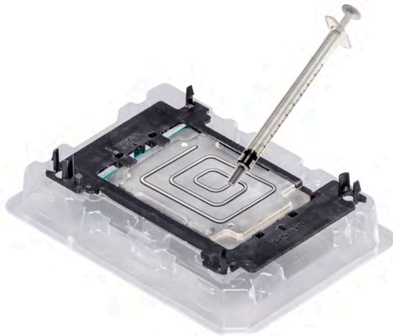
Figure 46. Applying thermal grease on top of the processor
