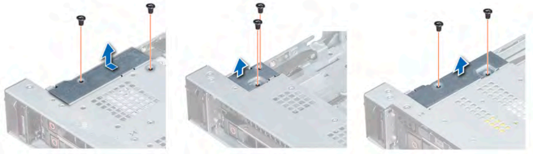
Figure 99. Removing the cable cover
