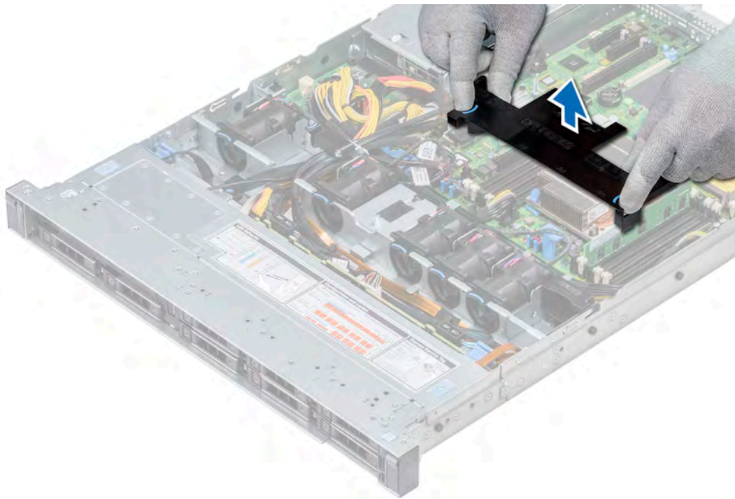
Figure 24. Removing the air shroud
