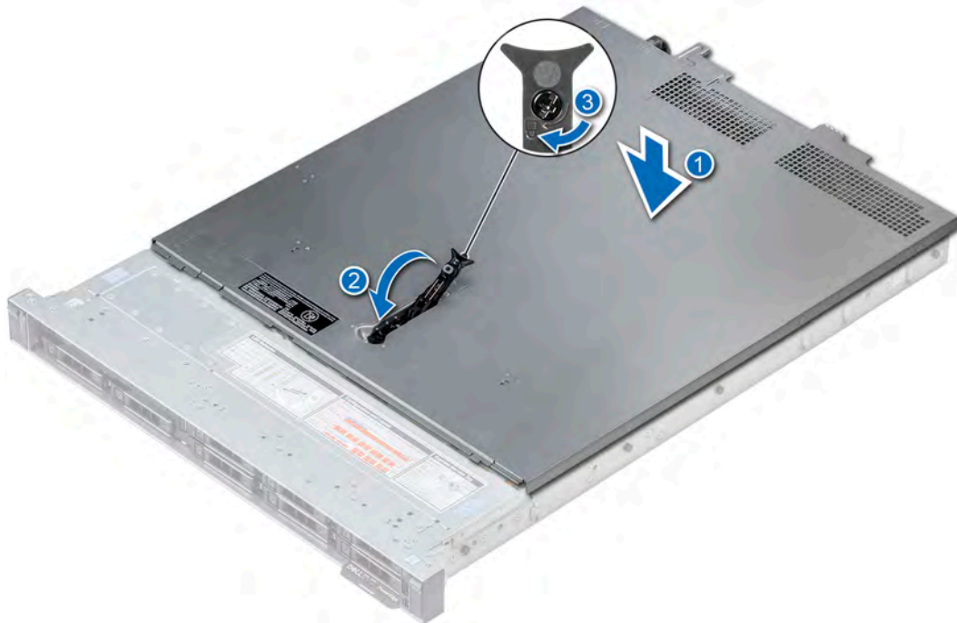
Figure 20. Installing the system cover
