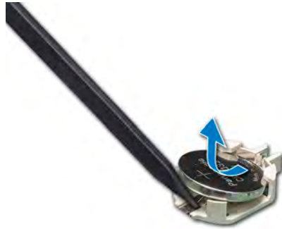
Figure 87. Removing the system battery
