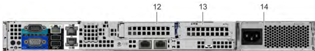
Figure 10. Back view of the system with 2 risers
