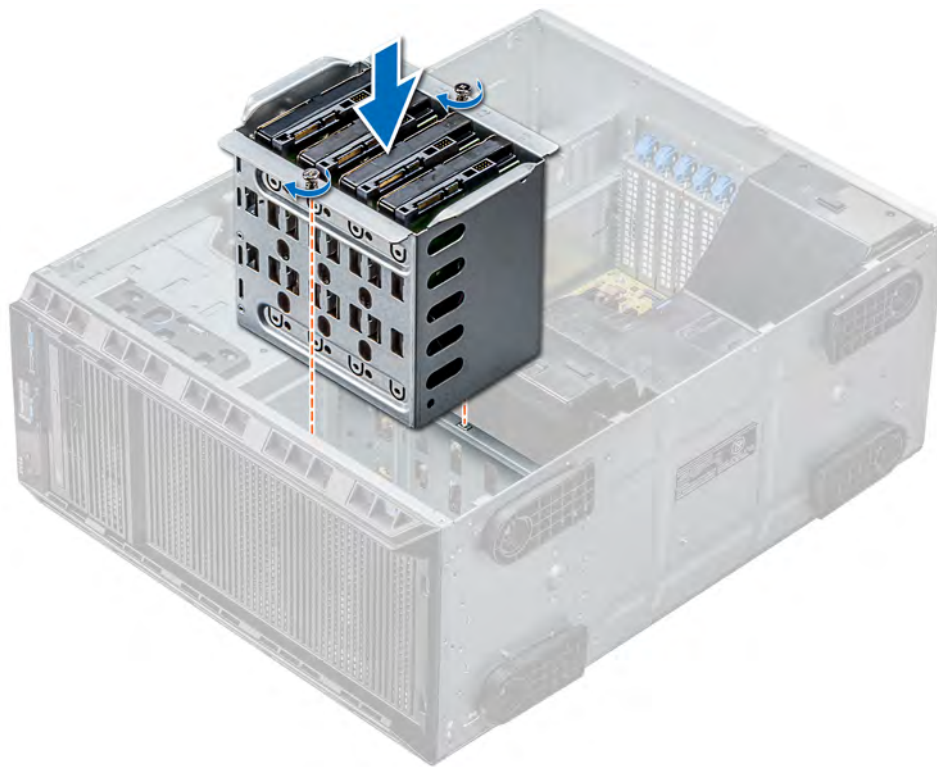
Figure 38. Installing the internal hard drive bay
