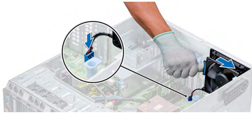
Figure 53. Installing the internal cooling fan
