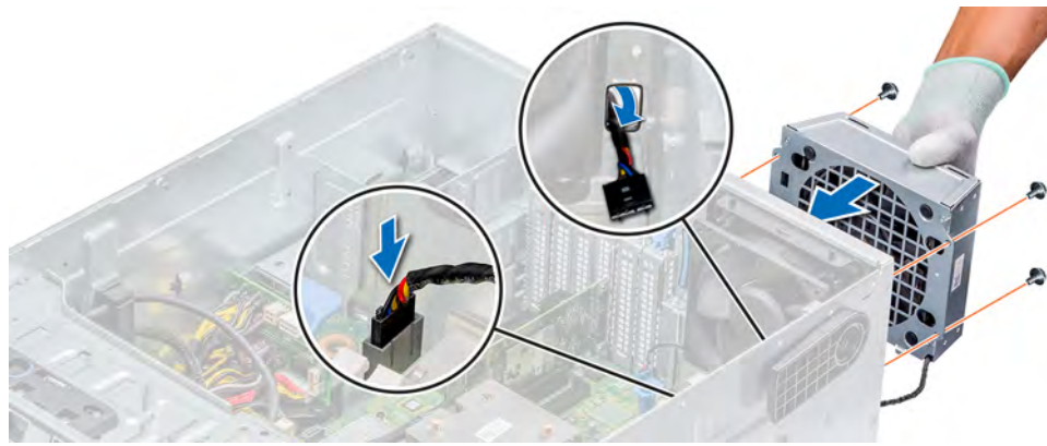
Figure 55. Installing the external cooling fan
