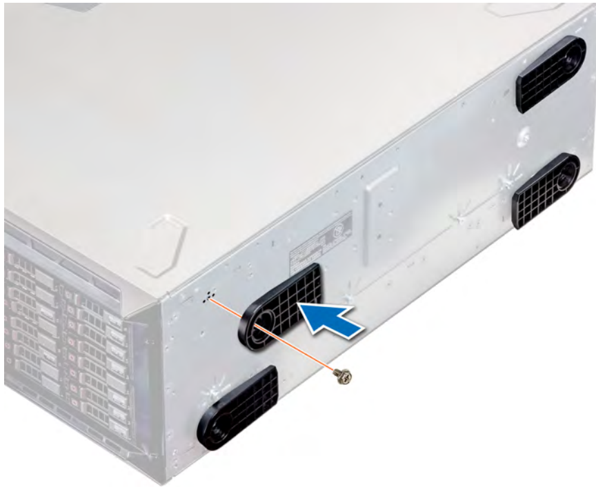
Figure 16. Installing the system feet
