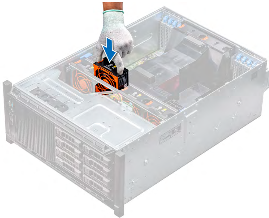
Figure 48. Installing a middle cooling fan
