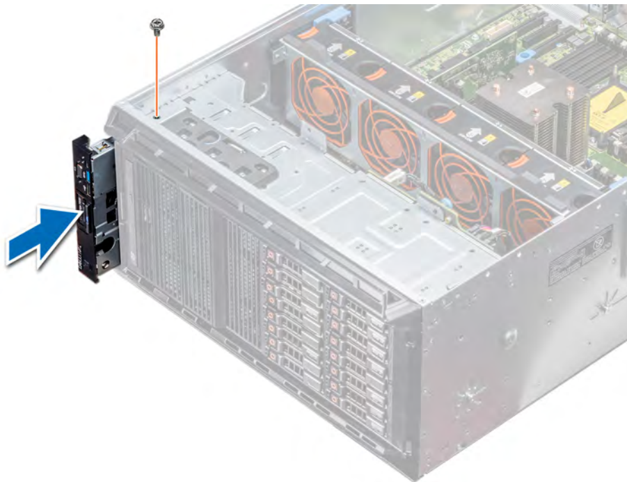
Figure 103. Installing the control panel assembly
