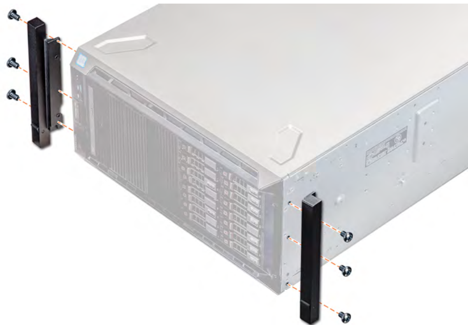
Figure 116. Installing the system ears
