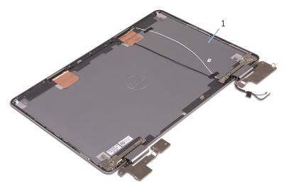
Figure 38. Display back-cover and antenna assembly
