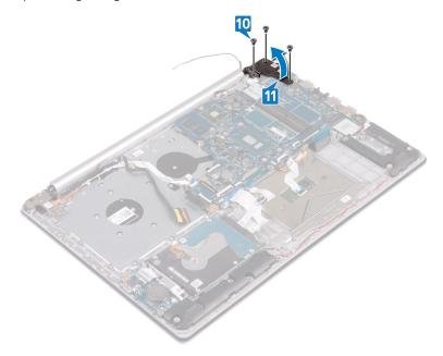
Remove the screw (M2x4) that secures the system board to palm rest and keyboard assembly.
