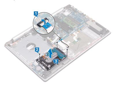
Disconnect the interposer from the hard-drive assembly.
